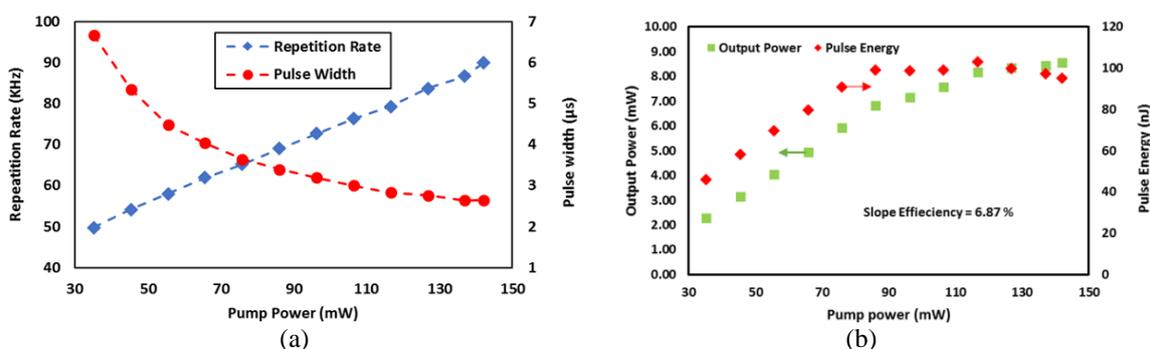
Fig. 4. Laser performance within 35 mW to 142.5 mW. (a) Repetition rate and pulse width. (b) Output power and pulse energy.
