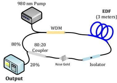
Fig. 2. Schematic illustration of the proposed GNPs based passive Q-switched EDFL.
