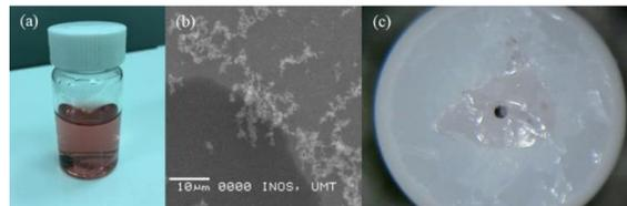
Fig. 1. GNPs characteristics. (a) Solution. (b) SEM image. (c) Film position on fiber ferrule.
