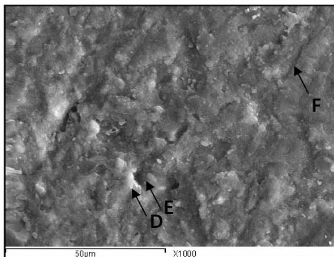
*Fig. 3 Scanning electron micrograph of In-ceram alumina specimen subjected to conventional glazing. D: refers to glazed patches, E: shows crater like irregularity and F: shows crack formation.*
