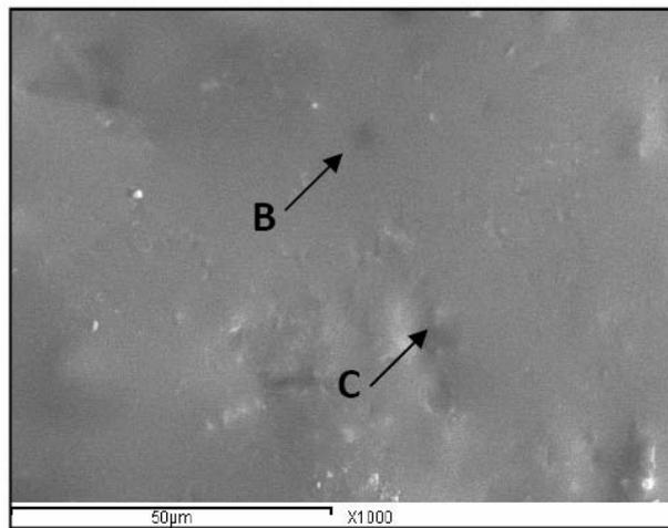
*Fig. 2: Scanning electron micrograph of porcelain specimen subjected to 6.2 Joule/cm<sup>2</sup> excimer laser glazing. B, C: refer to shallow splodgy areas of melting.*
