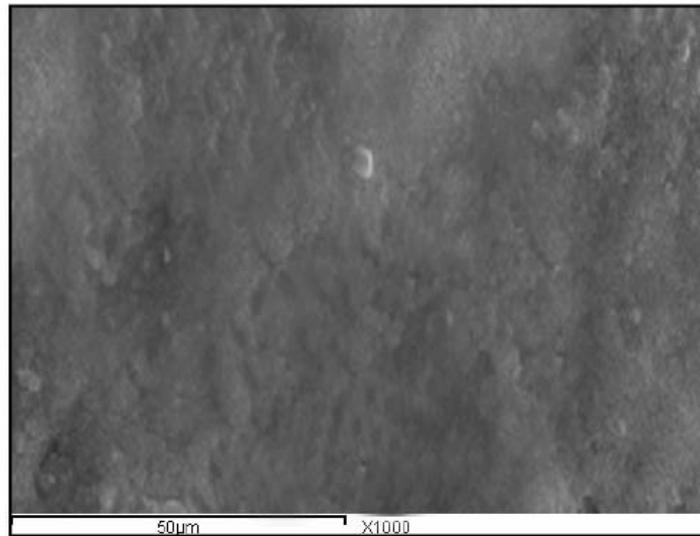
*Fig. 4: Scanning electron micrograph of In-ceram alumina specimen subjected to 10 watt CO<sub>2</sub> laser glazing.*
