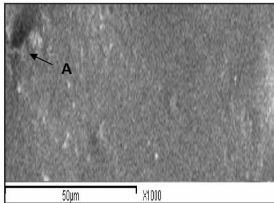
*Fig. 1: Scanning electron micrograph of porcelain specimen subjected to conventional glazing. A: Refers to large void formation.*
