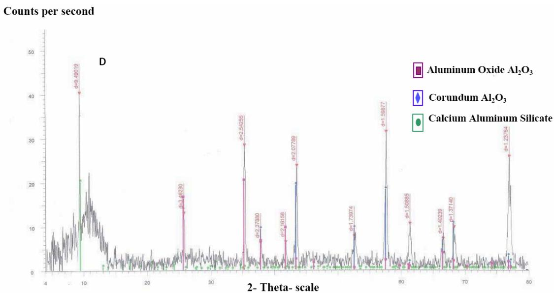
Fig. 6: Representative X-ray spectrum of In-Ceram Alumina specimens subjected to C: Conventional glazing, D: 6.2 Joule/cm<sup>2</sup> excimer laser glazing.
