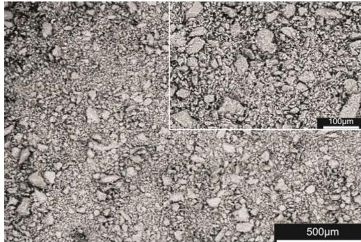
*Fig.7. Bone powder after final grinding, sorted by size before compaction*
