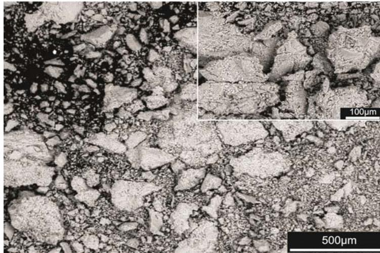
*Fig. 5. Bone powder after grinding for 10 minutes in ball mill*
