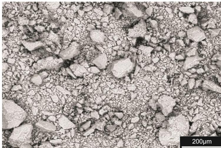
*Fig. 6. Bone powder after grinding for 60 minutes in ball mills*
