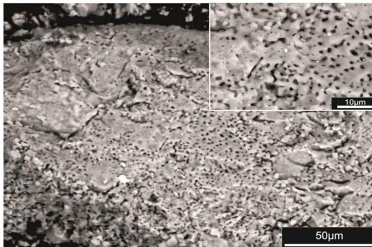
*Fig. 4. Sample after heat treatment at 300°C - most organic components from the constitution bone were removed (without water and collagen).*
