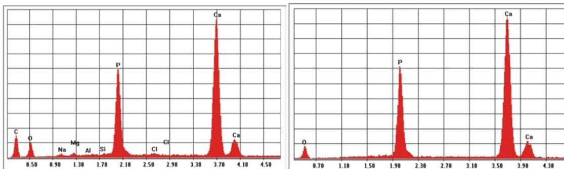
Fig.2. EDX spectra of bone mineral component from figure 1, with a Ca/P ratio = 1.688 (left) compared with analysis of standard samples of hydroxyapatite with a Ca/P ratio = 1.664 (right)
