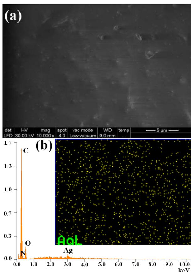
Fig. 1. SEM (a) and EDX(b) image of the polyurethane acrylates - silver film composite PUAc-8
