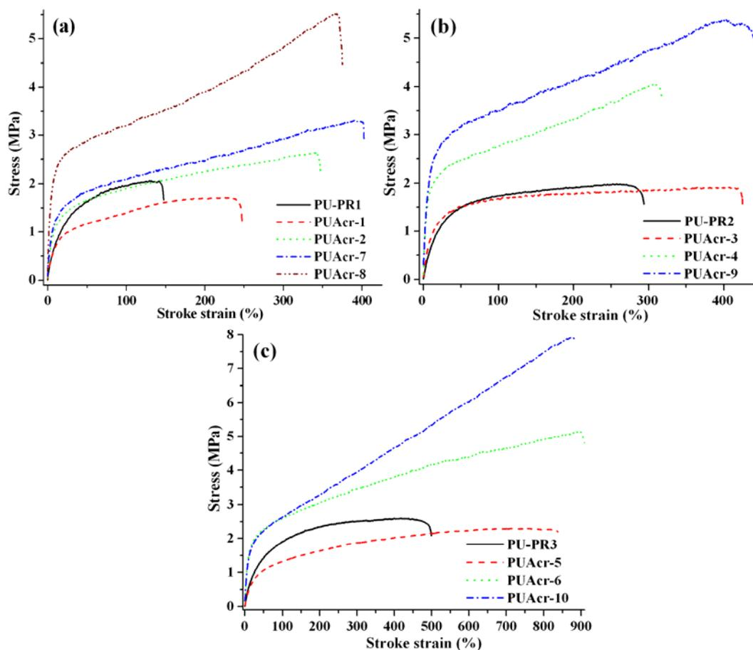
Fig. 3. Stress-strain curves for the polyurethane precursors, polyurethane acrylates and silver composites.
