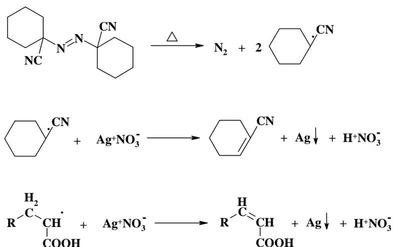
Scheme 3. The proposed mechanism for the reduction of silver cations by an electron transfer reaction
