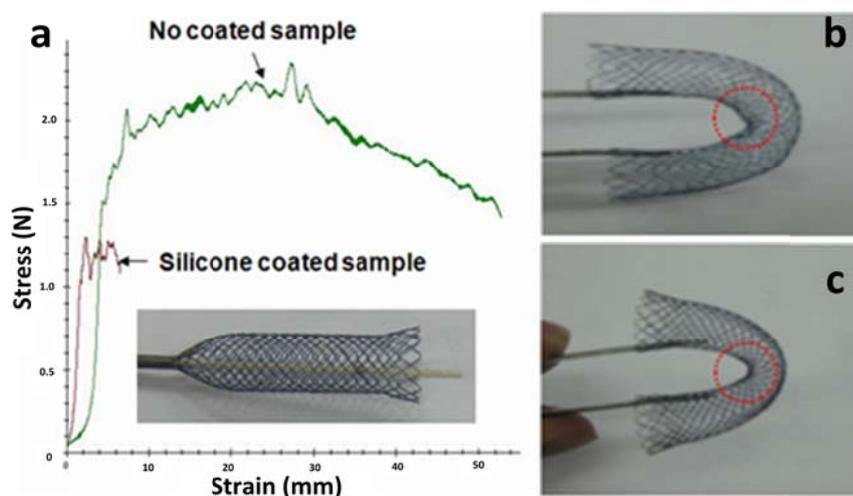
Fig. 4. (a) Depolyment/pull-out test graph of coated and bare stents; photographic images of (b) bare and (c) silicone-coated Nitinol stents after simple bending.
