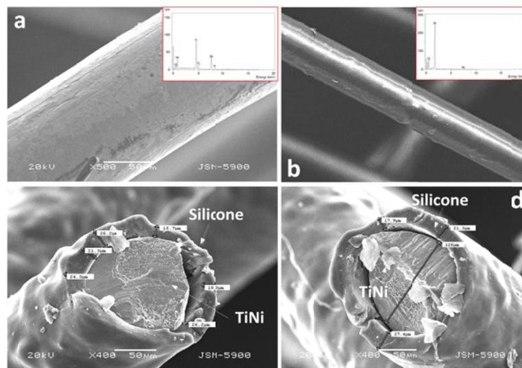
*Fig. 2. SEM and photographic images of bare and silicone-coated stents: (a) bare Nitinolstent (inset: EDS spectra); (b) silicone-coated Nitinolstent wire; cross-section of silicone-coated Nitinolstent wires cured at (c) 150°C, and (d) 200°C.*
