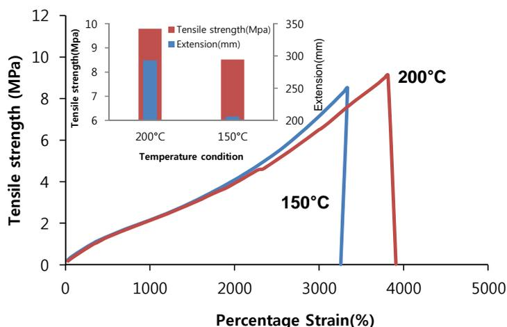
Fig 3. Stress-strain curves of the silicone film (without wire) cured at different temperatures.
