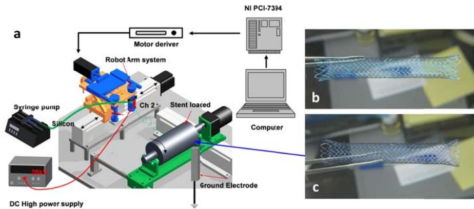
Fig. 1.(a) Electrospinning set-up, (b) bare (uncoated) Nitinol stent, and (c) Silicone-coated silicone Nitinolstent.
