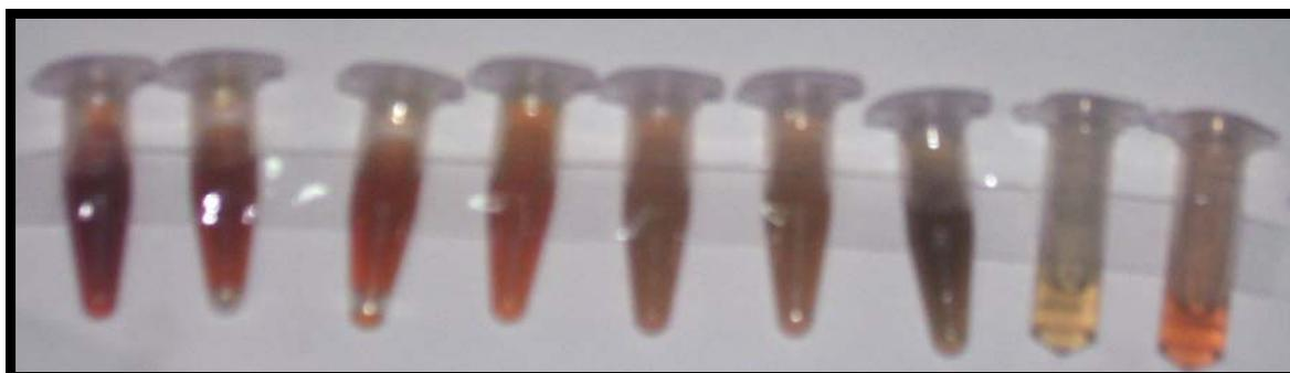
Fig. 1. Optical photograph of the colloidal solution of silver nanoparticles reduced by *Mentha Piperita* leaf extract with different concentrations.
