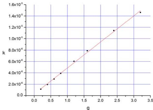
Fig. 7: Dependence of the crystallization rate as function of  $g$  for a cubic box with  $L = 5$  and growth velocity  $v = 0.01$ . The red line is the linear fit of data.
