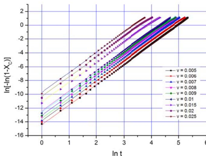
Fig. 4: Representation of the equation (6) for a cubic box with  $L = 5$  and concentration of nuclei  $g = 0.8$  for several growth velocities. The lines represent the individual linear fits for each set of data.
