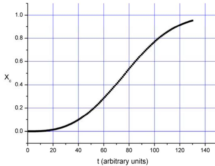
Fig. 2: Volume fraction of the polymer as function of time for a cubic box with  $L = 5$ , growth velocity  $v = 0.005$  and concentration of the nuclei  $g = 16$ .
