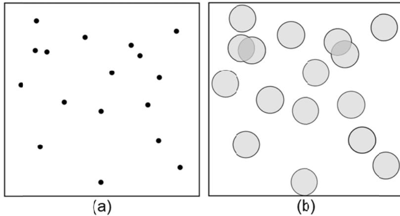
*Fig. 1: Mechanism of the instantaneous nucleation.
