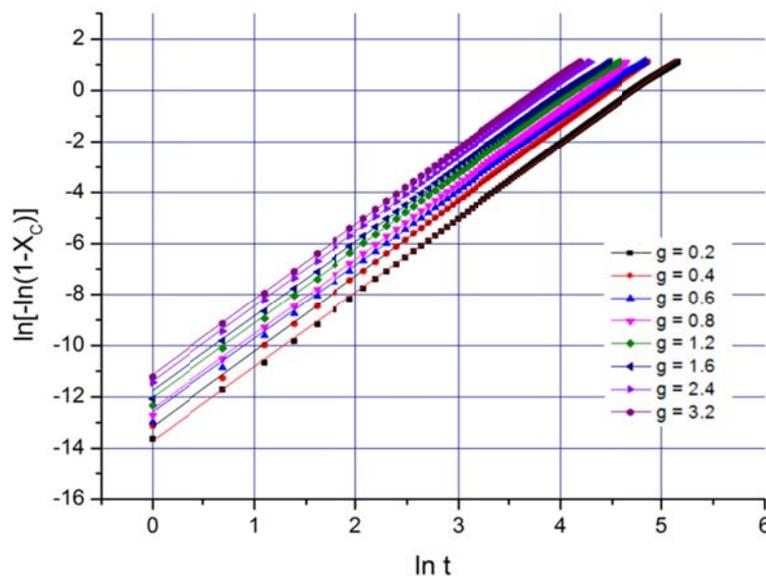
Fig. 6: Representation of the equation (6) for a cubic box with  $L = 5$ , growth velocity  $v = 0.01$  for several concentrations of the nuclei. The lines represent the linear fits for each set of data.
