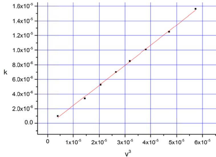
Fig. 5: Dependence of the crystallization rate as function of  $v^3$  for a cubic box with  $L = 5$  and concentration of nuclei  $g = 0.8$ . The red line is the linear fit of data.
