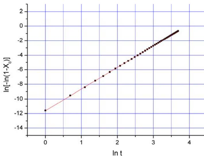
Fig. 3: Representation of the equation (6) for a cubic box with  $L = 5$ , growth velocity  $v = 0.005$  and concentration of the nuclei  $g = 16$ . The red line represents the linear fit of the data.
