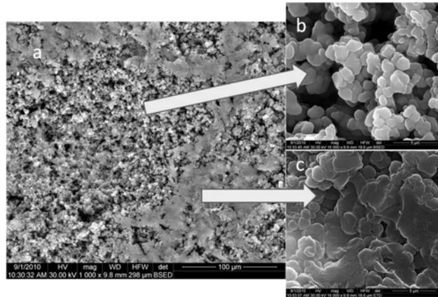
Fig.4. SEM morphology of sample A: a – general view at 1000x; b – detail of the Cas zone at 16000 x; c - detail of the PHEMA-coated Cas grains at 16000 x
