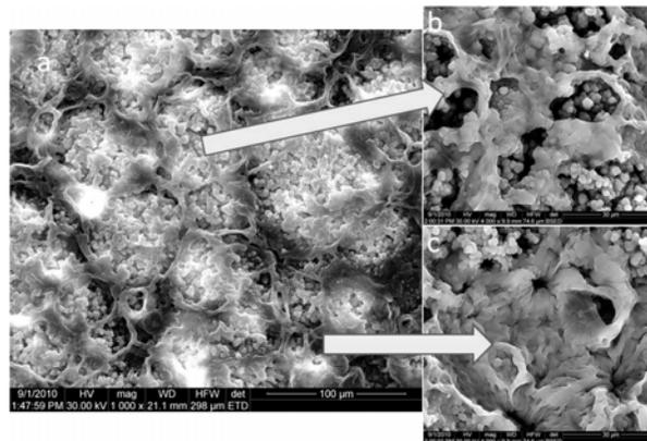
Fig.5. SEM morphology of a cross-section of sample E: a –general view at 1000x; b – detail of the Cas-PHEMA zone at 4000x; detail of a PHEMA richer zone at 4000x; few pores are also visible.
