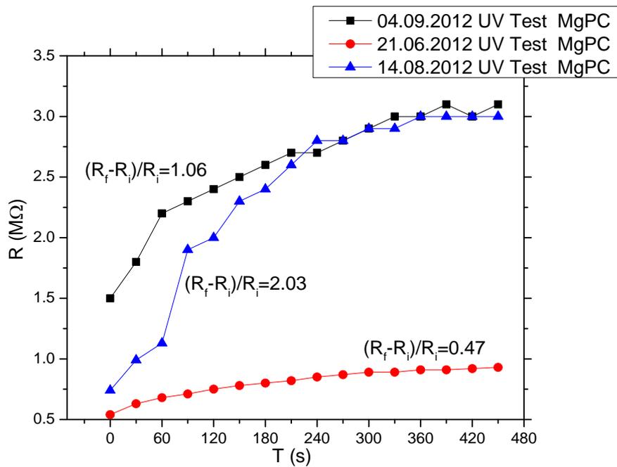
Fig.5. UV radiation effect on 5 Langmuir Blodgett thin layers sensor based on Mg – phthalocyanine, Barium stearate and carbon nanotubes for a period of time of three months ( $R_f$ = final resistivity,  $R_i$ = initial resistivity)
