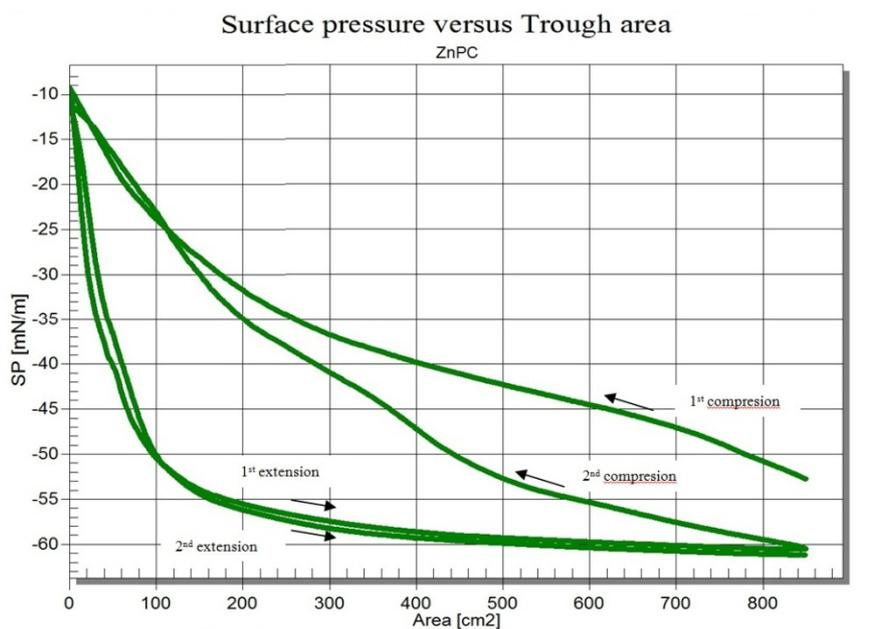
*Fig.3. The hysteresis curves, surface pressure versus area of Barium stearate and carbon nanotubes with Zinc phthalocyanine*
