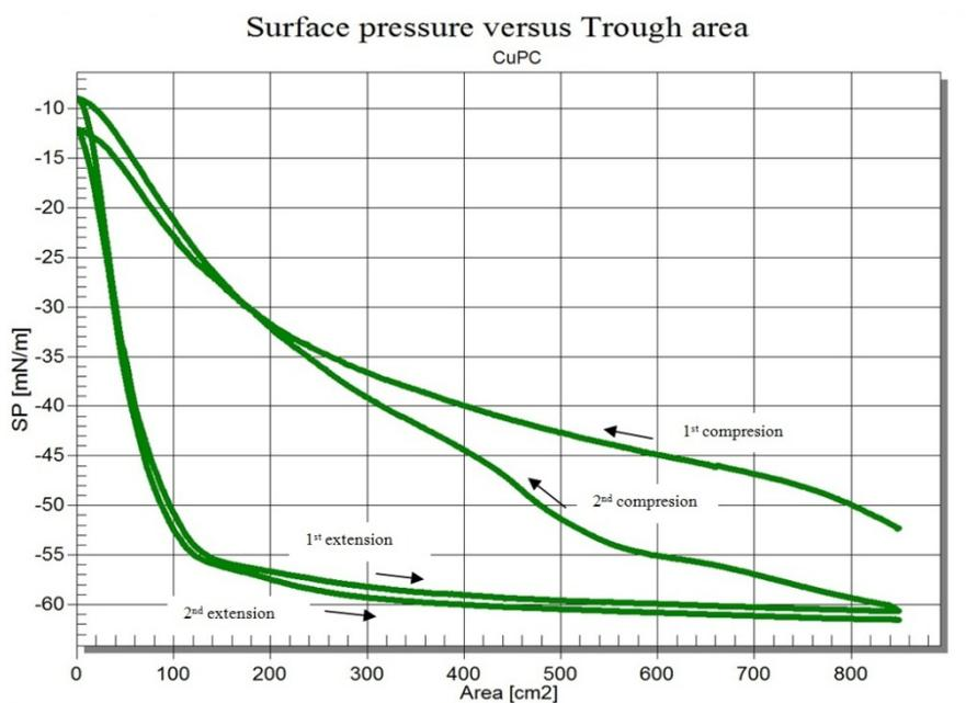
*Fig.2. The hysteresis curves, surface pressure versus area of Barium stearate and carbon nanotubes with Copper phthalocyanine*
