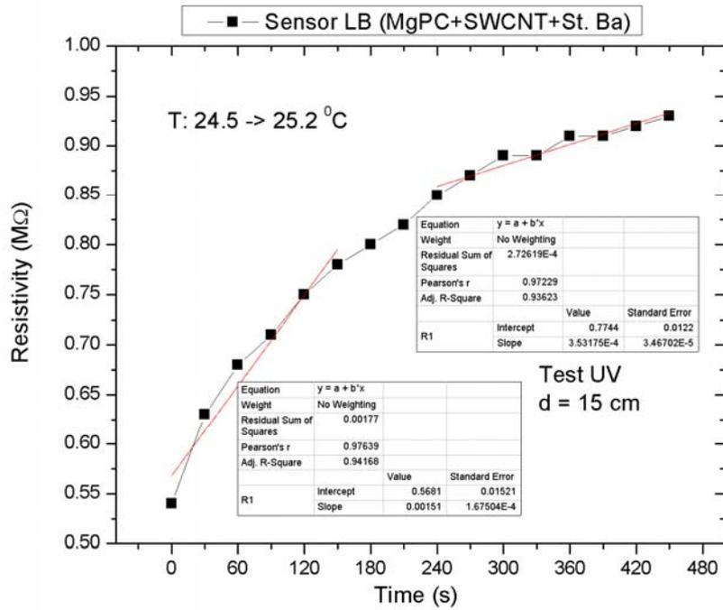
Fig.4 The effect of UV radiation of 5 Langmuir Blodgett thin layers sensor based on Mg – phthalocyanine, Barium stearate and carbon nanotubes
