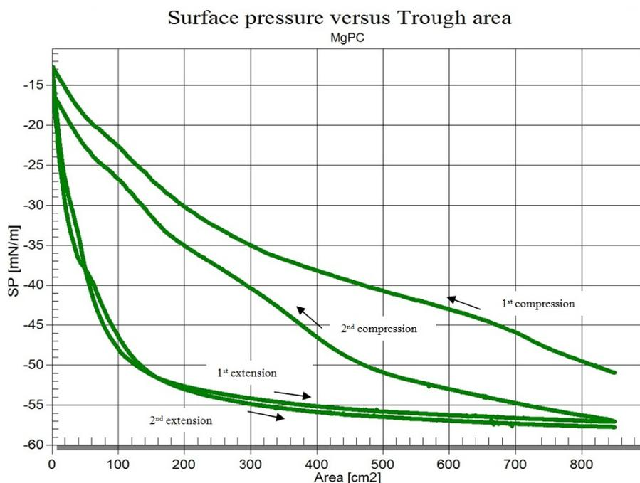
Fig.1. Shows the hysteresis curves, surface pressure versus area curves of Barium stearate and carbon nanotubes with Magnesium phthalocyanine
