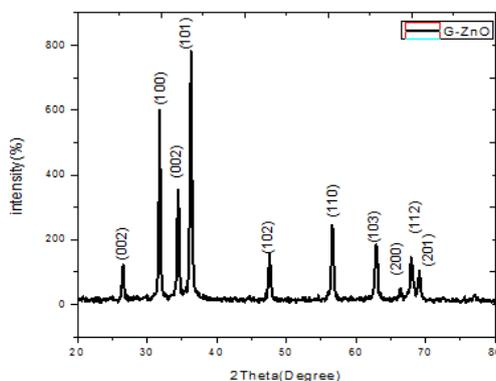
Fig. 1. XRD pattern of graphene oxide – ZnO nanocomposite.
