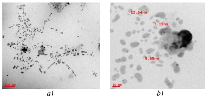
Fig. 5. TEM image of Graphene-ZnO nanocomposite (a) 100nm (b) 20nm.
