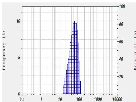
Fig. 7. Particle distribution in the dynamic light scattering of graphene oxide –ZnO nanocomposite.
