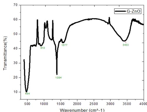
Fig. 3. FTIR spectrum of graphene Oxide - ZnO nanocomposite.
