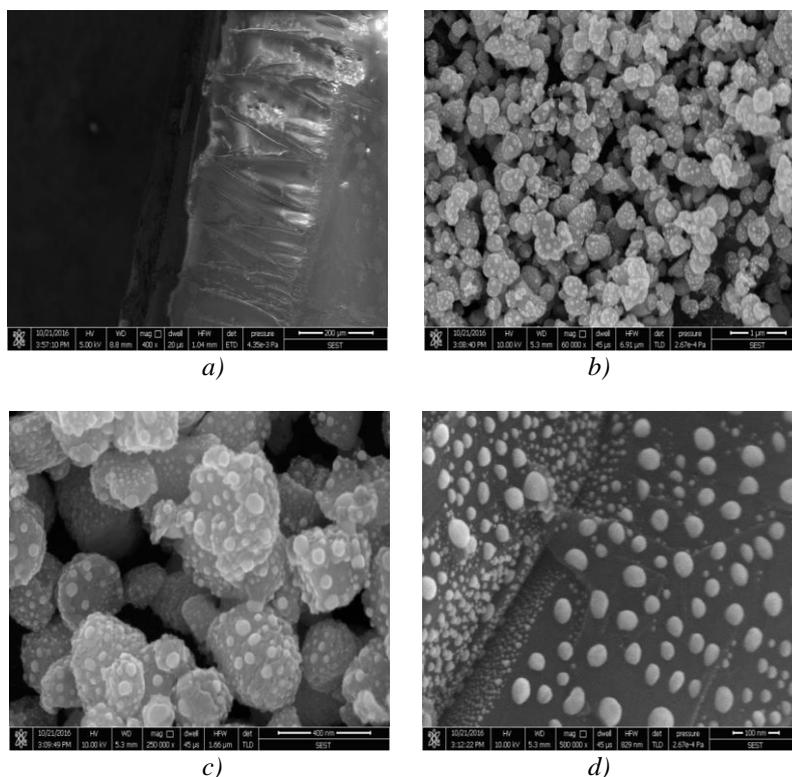
Fig. 4. FESEM image of Graphene oxide - ZnO nanocomposite (a) 20 μm (b) 1 μm (c) 400 nm and (d) 100 nm.
