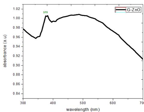
Fig. 2. UV absorbance spectrum of Graphene oxide –ZnO nanocomposite.
