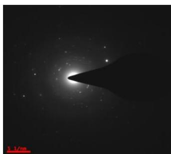
Fig. 6. SAED pattern of Graphene-ZnO nanocomposite.
