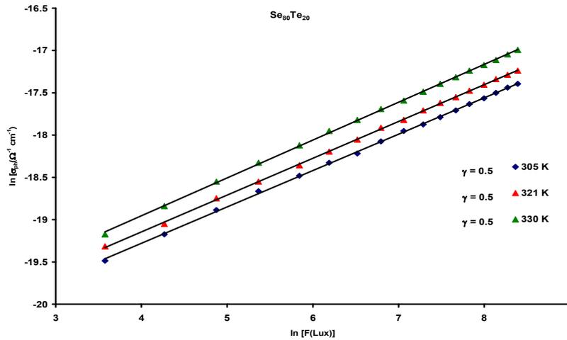
Fig. 3. Intensity dependence of photoconductivity at various temperatures in  $\text{a-}\text{Se}_{80}\text{Te}_{20}$ .
