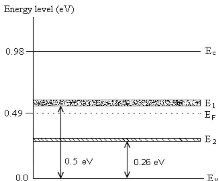
Fig. 5. Energy level diagram for defect states in the mobility gap of a-Se<sub>80</sub>Te<sub>10</sub>Cd<sub>10</sub> thin films at a particular intensity of light 1190 Lux.
