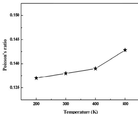
Fig. 4. The Poisson's ratio of graphene sheets subjected to the tensile loading at different temperatures.
