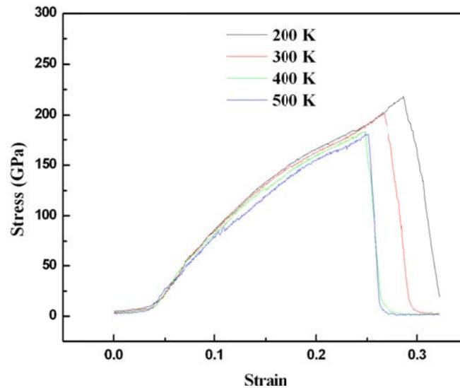
Fig. 3. The stress-strain curve of graphene sheets subjected to the tensile loading at different temperatures.
