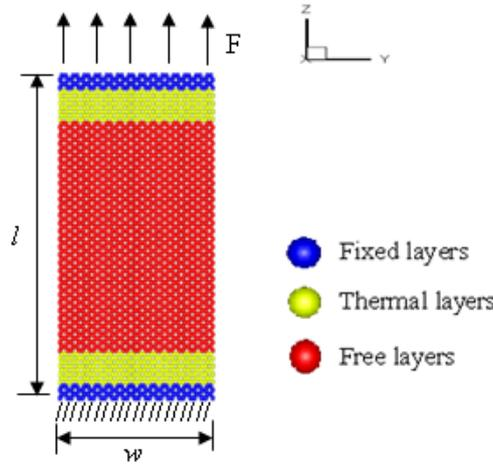
Fig. 1. Schematics of MD of graphene sheets subjected to a uniaxial tensile loading.
