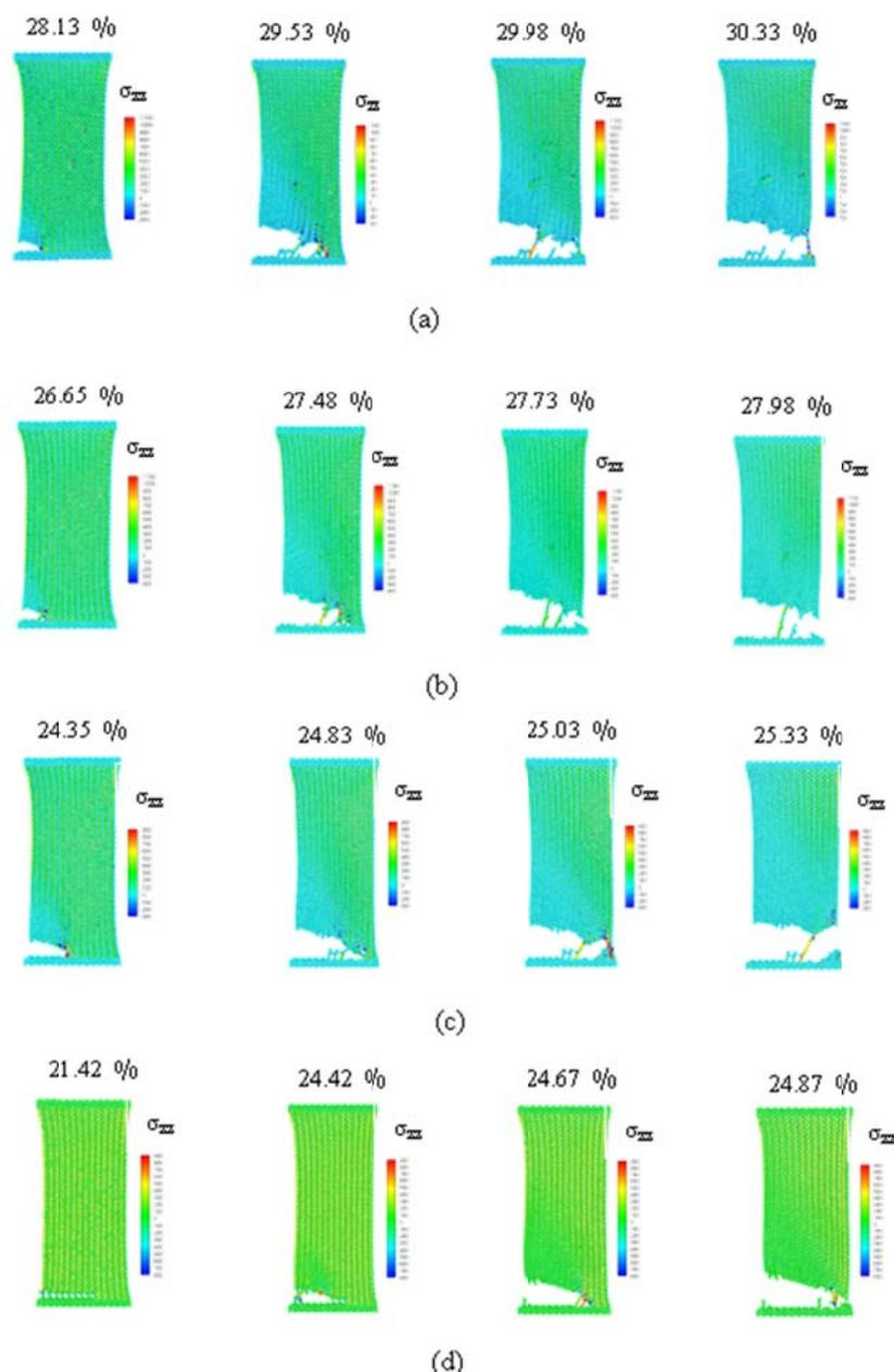
Fig. 2. The snapshots of graphene sheets induced a tensile stress until failure at temperatures of (a) 200K, (b) 300K, (c) 400K, and (d) 500K.
