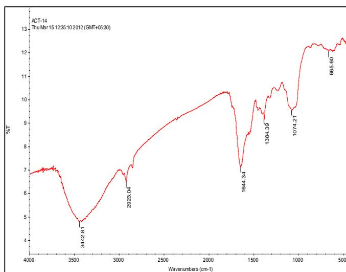
Fig. 3 FTIR spectrum of *Streptomyces sp. VSMGT1014* mediated AgNP's
