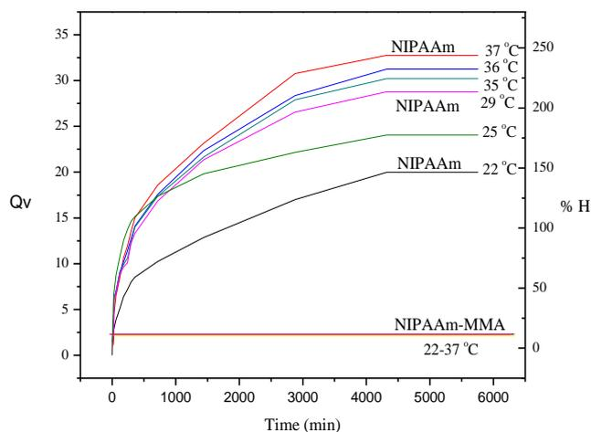
Fig. 3. Behavior of the degree of crosslinking  $Q_v$ , the percentage of moisture %H NIPAAm hydrogel and (NIPAAm-MMA) gel
