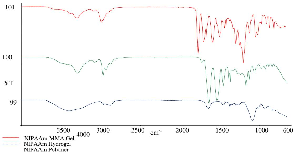
Fig. 2. FT-IR of the polyNIPAAm, NIPAAm hydrogel and NIPAAm-MMA gel
