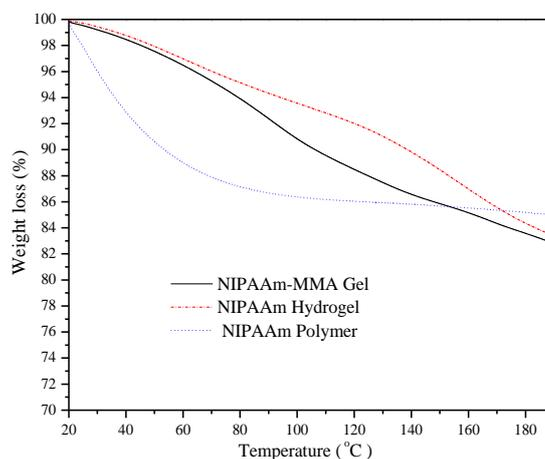
Fig. 4. TGA of NIPAAm hydrogel, (NIPAAm-MMA) gel and NIPAAm polymer
