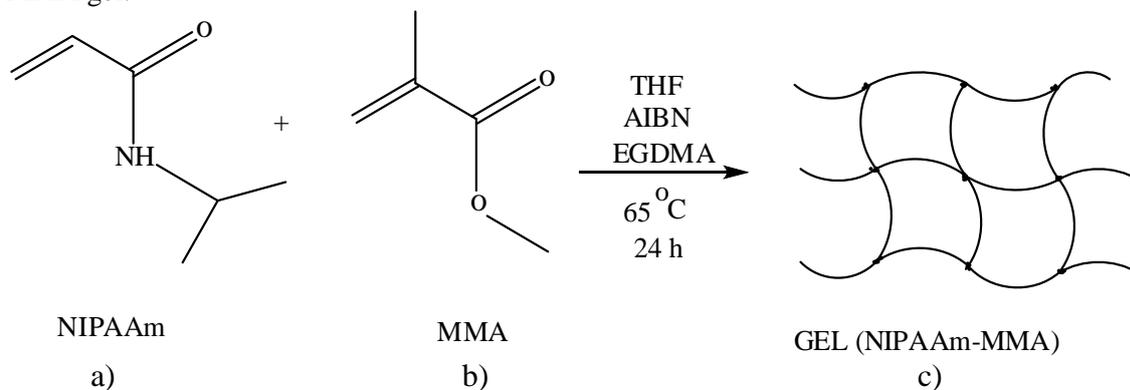
Fig. 1. Scheme of the reaction of (NIPAAm-MMA) copolymer gels
