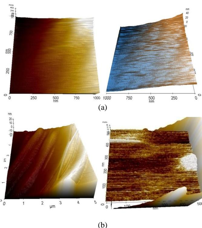
Fig. 5. AFM micrographs of hydrogel of NIPAAm (a) gel of NIPAAm-MMA (b)
