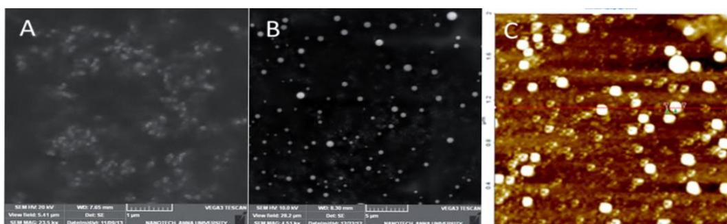
Fig. 1 (A) SEM image showing spherical shaped CHIT-NPS (B) SEM image showing spherical shaped QUER-CHIT nanoparticles (C) AFM image showing well-defined spherical shaped QUER-CHIT nanoparticles
