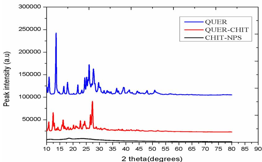
Fig 2. XRD Spectra of pure QUER, QUER-CHIT and CHIT nanoparticles
