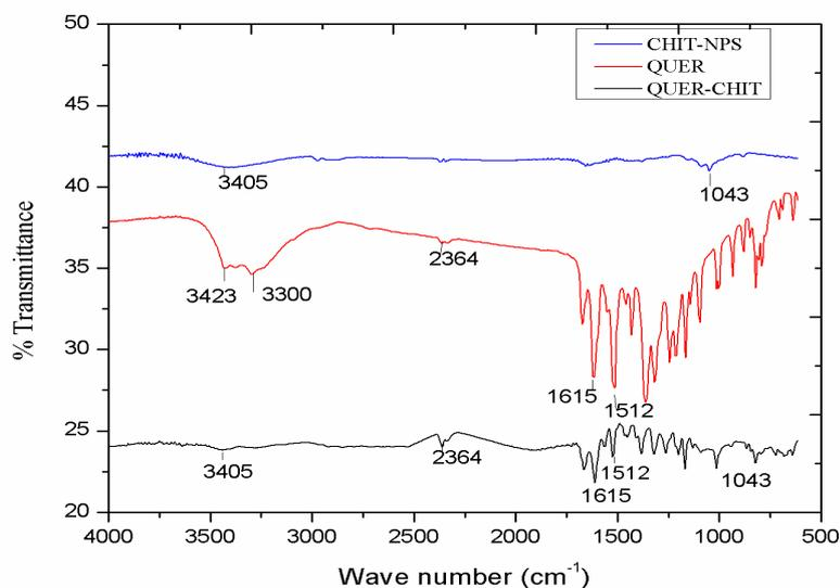
Fig. 3 FT-IR Spectra of QUER, QUER-CHIT and CHIT nanoparticles
