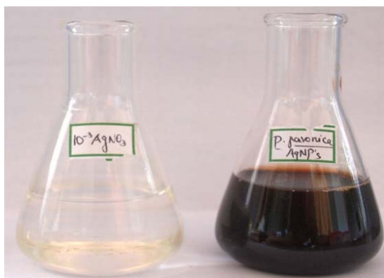
Fig. 1. Erlenmeyer flasks containing bio-synthesized silver nanoparticles by Padina pavonica , before reaction (left) after reaction (right)
