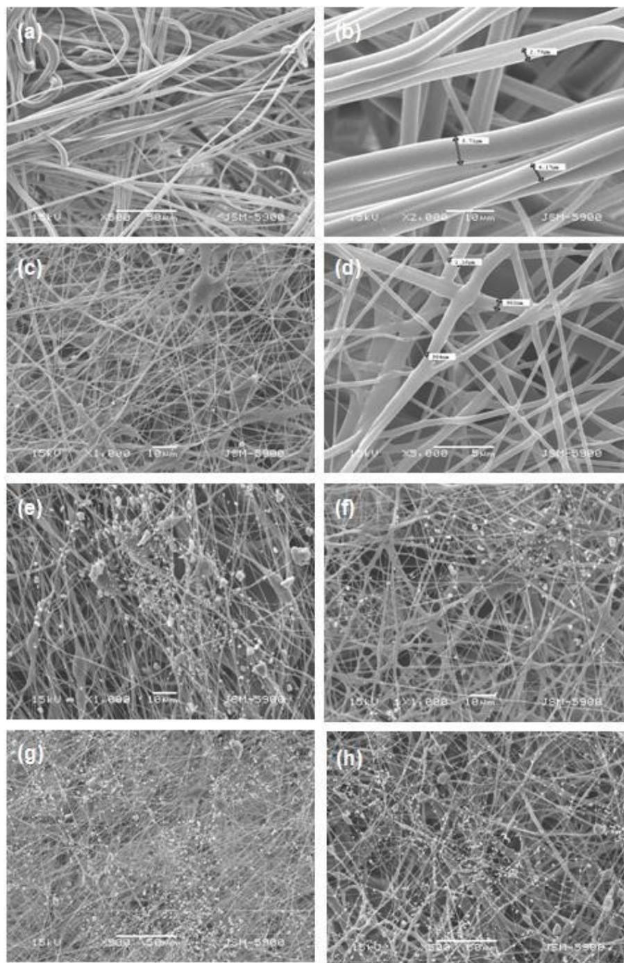
*Fig. 3 FESEM images (a)(b) nonwoven fabric (c)(d) Air filter composite T-5min (e) Air filter composite T-10min (f) 15min (g) Air filter composite Y-axis-150 mm (h) Air filter composite Y-axis-200 mm*
