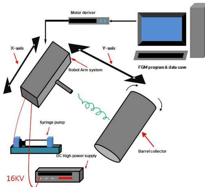
Fig. 1 Electrospinning system FGM technology mimetic diagram.
