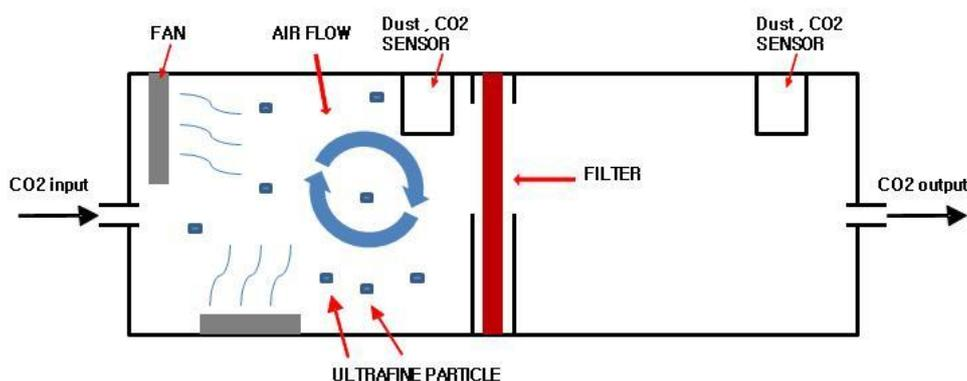
Fig. 2 Air Filtration Test Chamber Schematics
