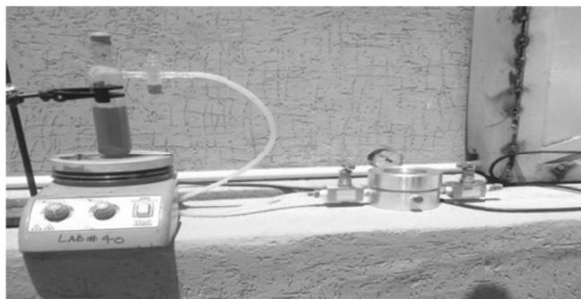
Fig. (8). Transferring of gaseous mixture from Schelling tube to evacuated reactor.
