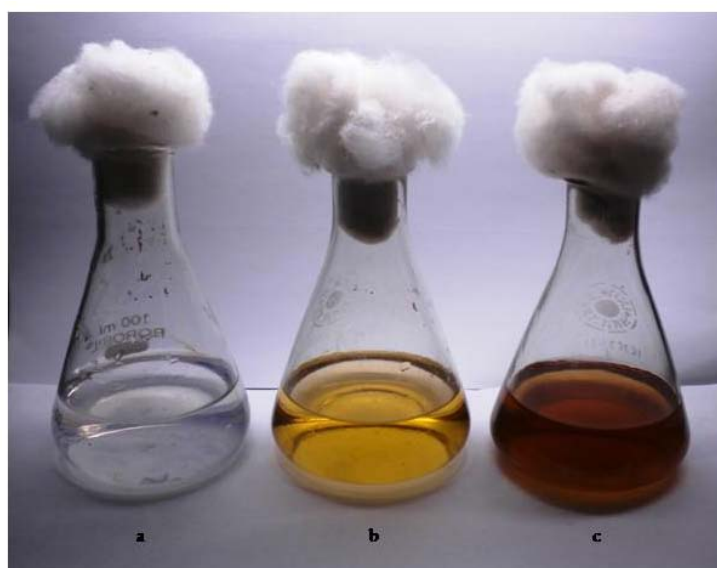
Fig. 1 Mycelia free culture filtrate showing color change (c) on addition of 1 mM \text{AgNO}_3 . No change in color observed in (a) negative and (b) positive controlled sets.
