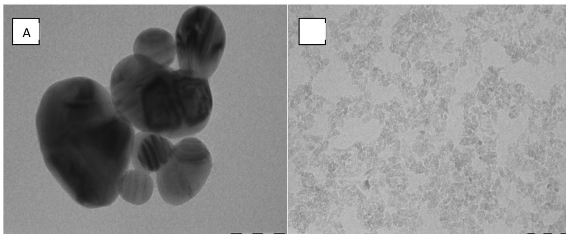
Fig. 5. (A & B) TEM images of Ag and TiO<sub>2</sub> NPs
