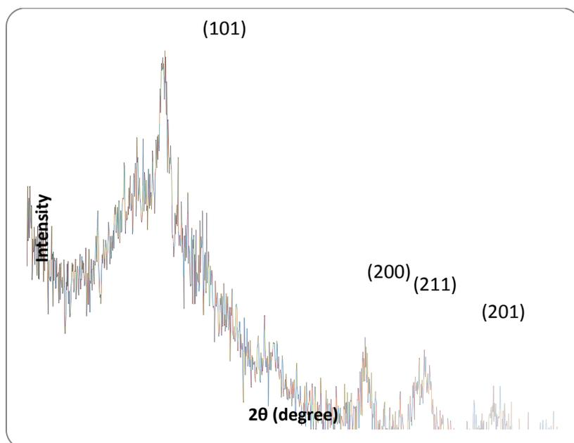
*Fig. 3. XRD pattern of TiO<sub>2</sub> NPs*
