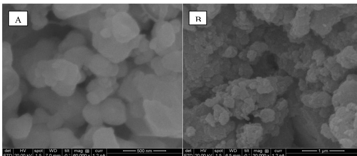
*Fig.4. (A & B) SEM images of Ag and TiO<sub>2</sub> NPs*
