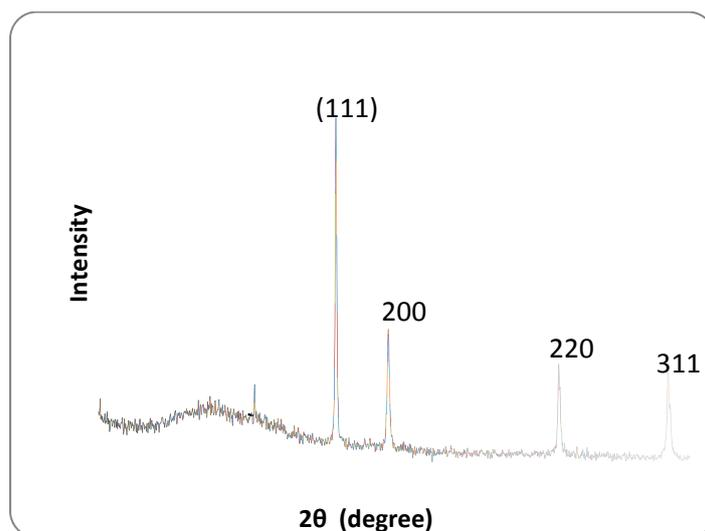
Fig. 2. XRD pattern of Ag NPs
