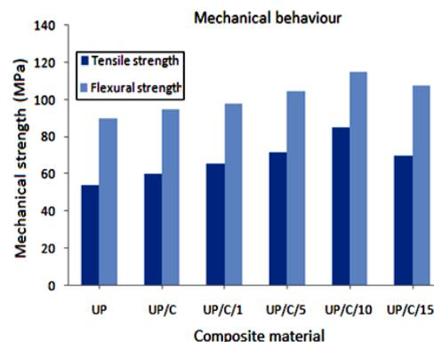
Fig. 7. Mechanical behaviour of composites.
