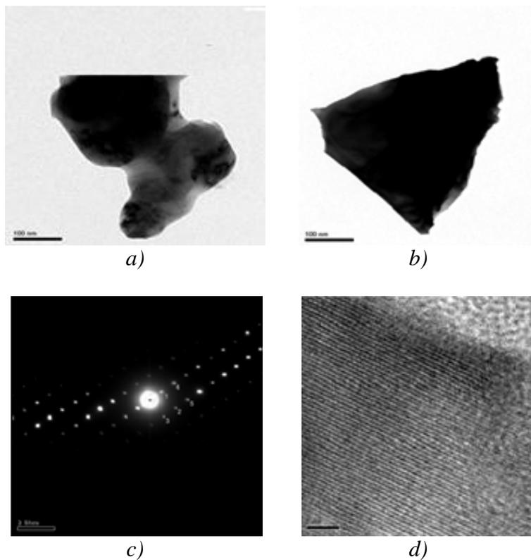
*Fig. 1 TEM images of (a & b) fine Cu particles, (c) selected area diffraction and (d) HR-TEM image of Cu confirming high crystalline pattern.*
