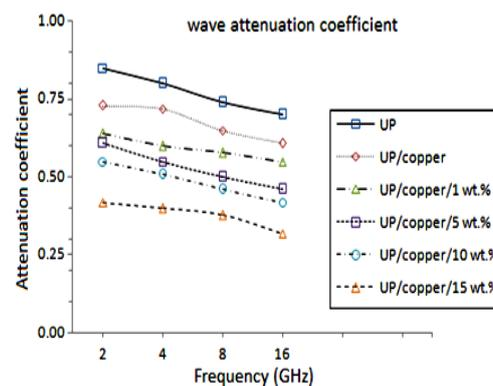
Fig. 5. Wave attenuation coefficient of composites in variable frequencies.
