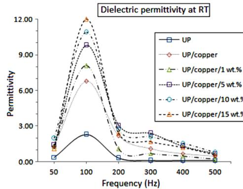
Fig. 4. Dielectric permittivity of copper wire-mesh and copper particle composites.
