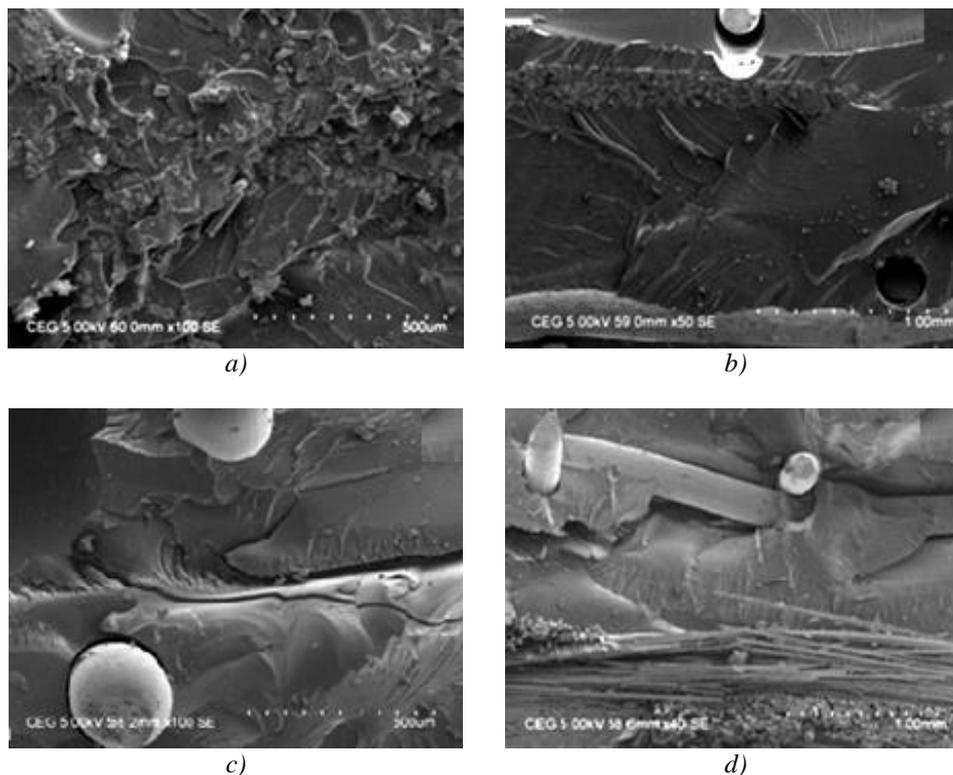
Fig. 8. SEM images of copper wire-mesh reinforced UP composites.
