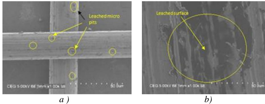
Fig. 3 Bleached surfaces of copper micro wire-mesh after acid etching.
