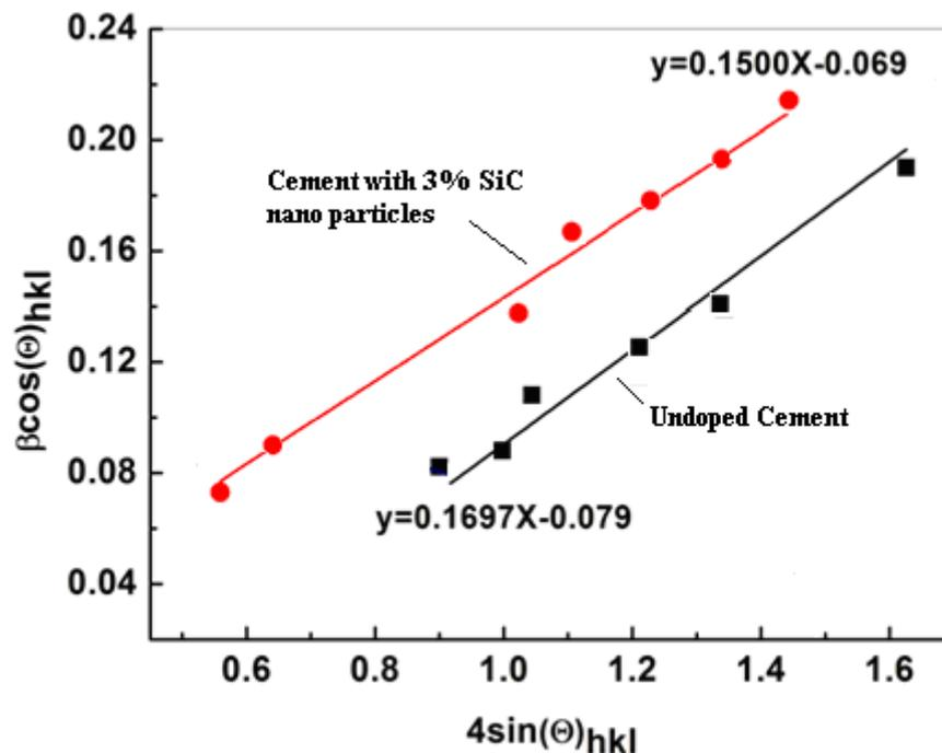
Fig. 13. The Williamson – Hall method based on X- Powder findings shows linear diagrams of  $\beta \cos\theta$  versus  $4\sin\theta$ .
