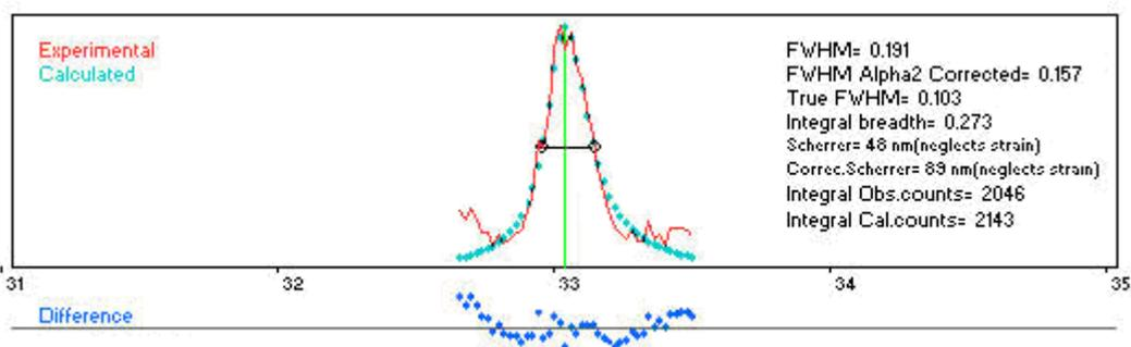
Fig. 3 -The size of SiCnanocrystallite (corresponding to figure 1) is appraised by X-powder method. It is shown that the typical diameter is of 48 nm.
