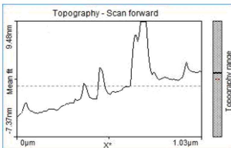
Fig. 11. AFM topographical images of synthesized cement mortar with 3% SiCnano particles at  $300^{\circ}\text{C}$  at  $\text{pH} = 8$ . The scan size was  $25.12 \text{ } \mu\text{m}^2$ .  $S_a$  of the synthesized SiCnanocrystallites is about  $7.121 \text{ nm}$  at  $\text{pH} = 8$ .
