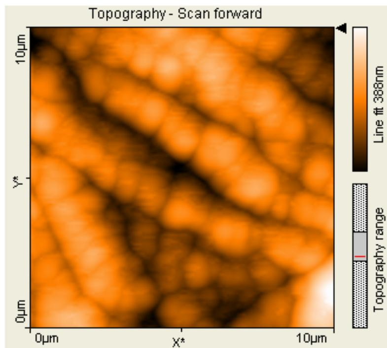
Fig. 6. Microscopy and surface morphology analyses of cement mortar with 3% SiC nano particles prepared at 300<sup>0</sup>C and performed by using AFM technique.
