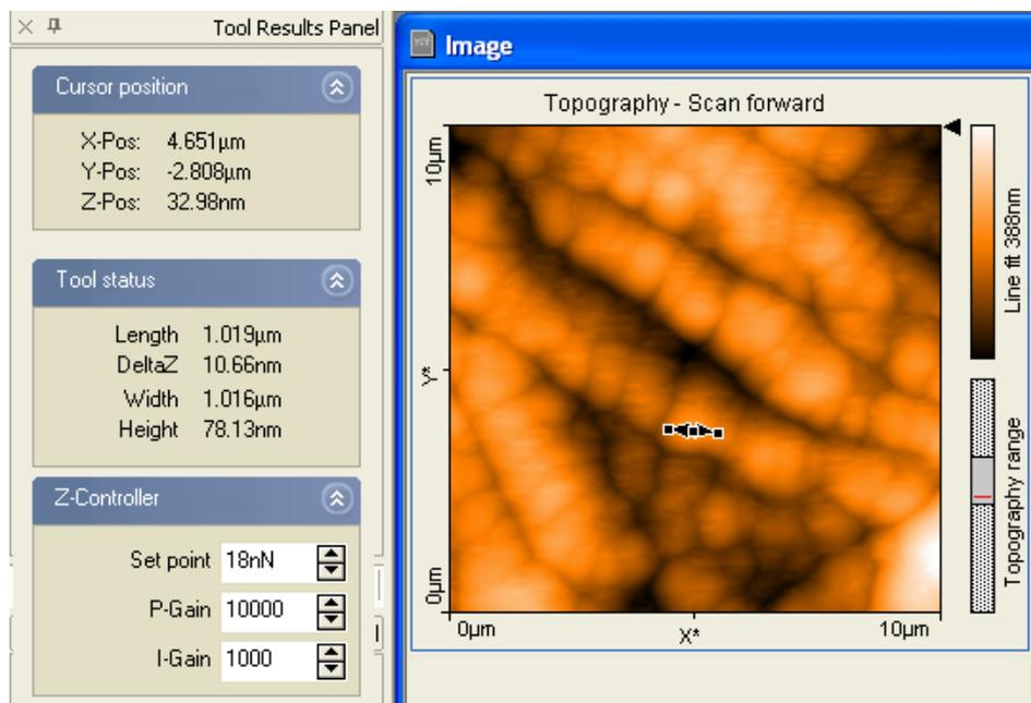
Fig. 8. Dislocation study of the cement mortar with 3% SiC nano particles prepared at 300°C by using the Nanosurf (see closed square) technique and the results of stress and strain are shown in the left hand side of the AFM image. The SiC crystallite length of the cement is 1019 nm.
