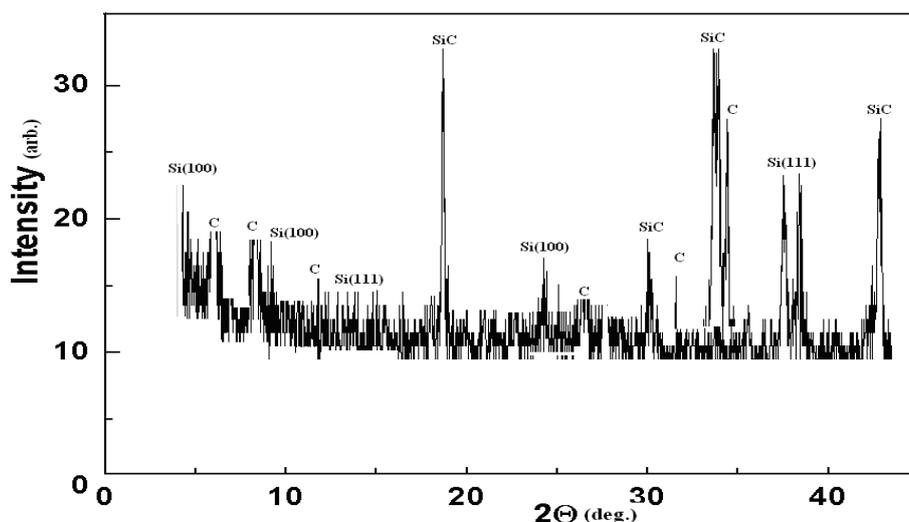
Fig. 1. The crystal phases of the mortar cement nanocrystallites were synthesized at  $300^\circ C$  and identified by XRD analysis. The Miller indices are not clear due to the cement structure. There are no significant peaks after  $40^\circ$  and we eliminated these peaks.
