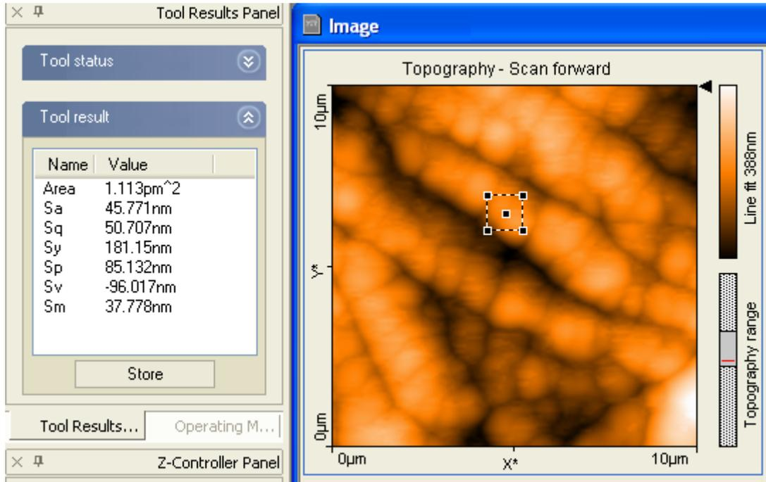
Fig. 9. Dislocation study of the cement mortar with 3% SiC nano particles prepared at 300°C by using the Nanosurf (see closed square) technique and Williamson-Hall data for stress and strain are shown in the left hand side of the AFM image.
