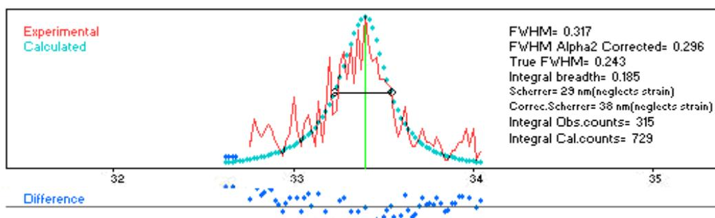
Fig.4- The size of SiCnanocrystallite (corresponding to figure 2 at 300°C) is appraised by X-powder method. It is shown that the typical diameter is of 29 nm.
