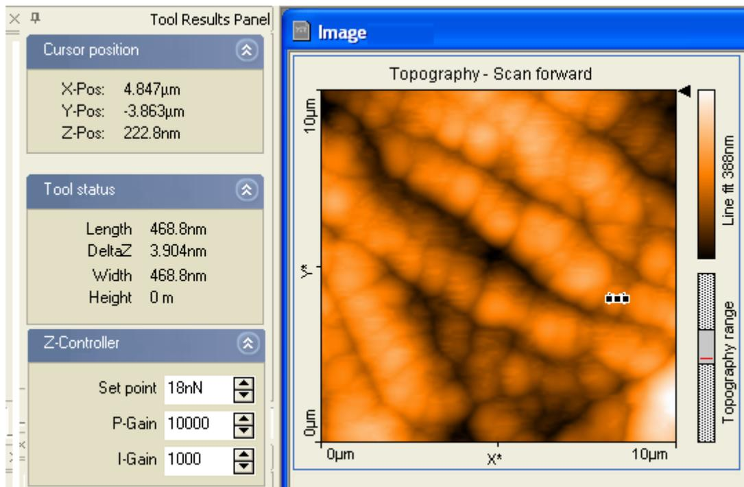
Fig. 7. Dislocation study of the cement mortar with 3% SiC nano particles prepared at 300°C by using the Nanosurf (see closed square) technique and the results of stress and strain are shown in the left hand side of the AFM image. The SiC crystallite length of the cement is 468.8 nm.
