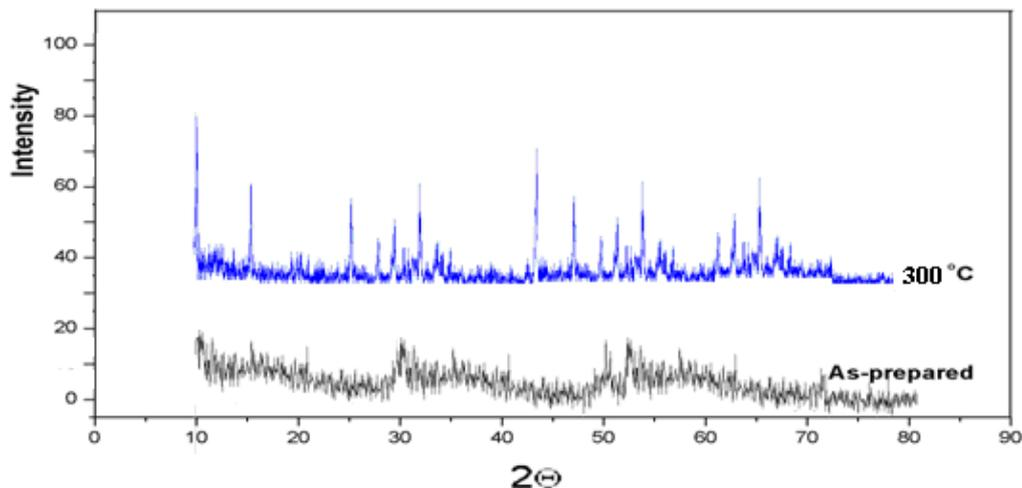
Fig. 2.The crystal phases of the cement mortar with 3% SiCnanocrystallites were synthesized at room temperature (down) and 300°C (up) and identified by XRD analysis.
