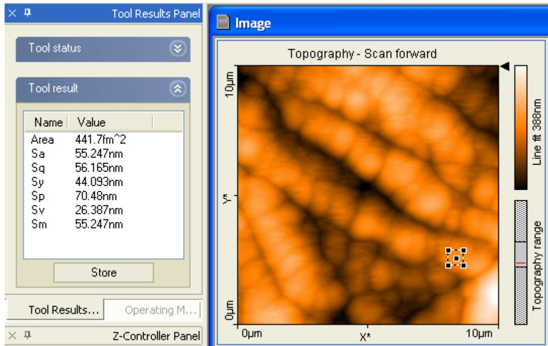
Fig. 10. Dislocation study of the cement mortar with 3% SiC nano particles prepared at 600°C by using the Nanosurf (see closed square) technique and Williamson-Hall data for stress and strain are shown in the left hand side of the AFM image.
