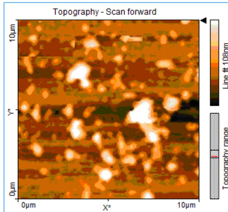
Fig. 5 -Microscopy and surface morphology analyses of cement prepared at 300<sup>0</sup>C and performed by using AFM technique.
