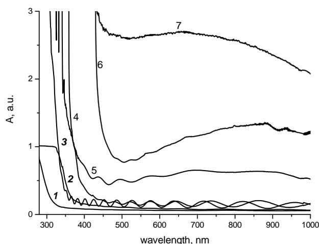
Fig. 1. Absorption spectra of ZrO<sub>2</sub> (1), TiO<sub>2</sub> (2), TZ2 (3), TZ1 (4), TZ7 (5), TZ3 (6), and TZ4 (7) films
