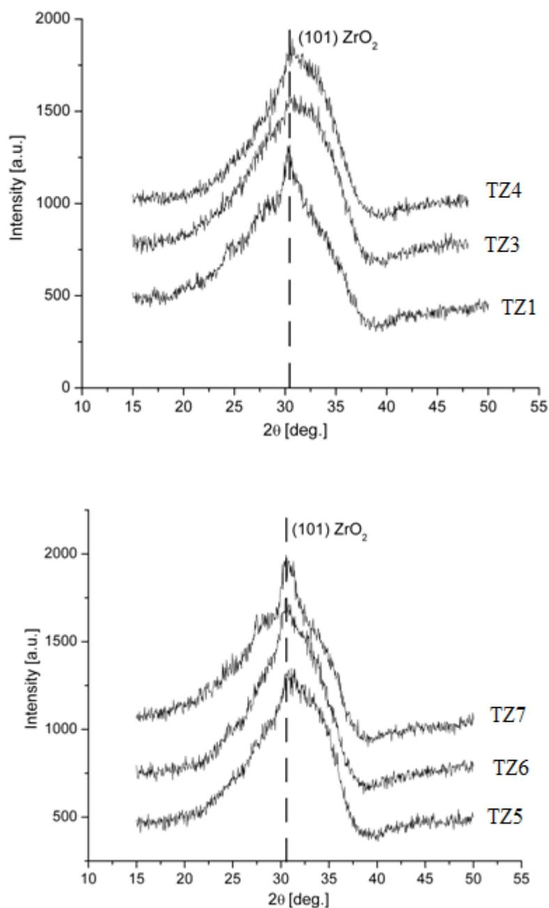
Fig. 2. XRD spectra of deposited TiO<sub>2</sub>/ZrO<sub>2</sub> thin films
