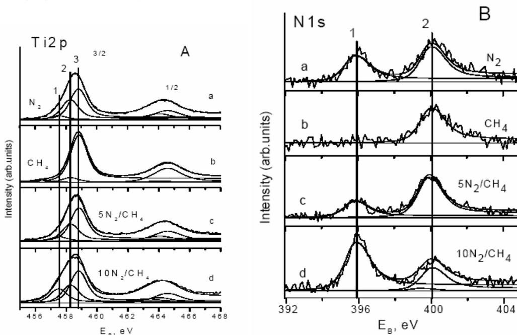
Fig. 3. XPS spectra of  $Ti2p$  (A) and  $N1s$  (B) energy for the samples TZ3 (a), TZ6 (b), TZ7 (c), TZ5 (d).
