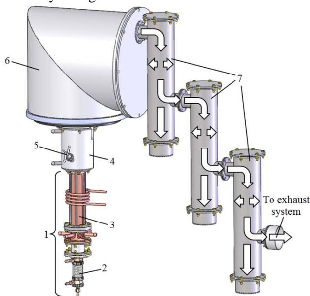
Fig. 1 - Scheme of the technological process of fine powder and nanopowder materials production: 1 – combined plasma torch; 2 – DC part of the combined plasma torch; 3 – RF part of the combined plasma torch; 4 – evaporating chamber (reactor); 5 – powder feeding tube; 6 – condensing chamber; 7 – trap modules
