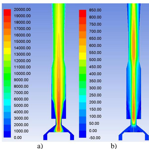
Fig. 4 – Results of calculation for arc plasma torch (arc voltage is  $U=70$  V, power in plasma is  $P=14.5$  kW, argon flow rate is  $G=25.9$  slpm): a – temperature, K; b – axial velocity, m/s
