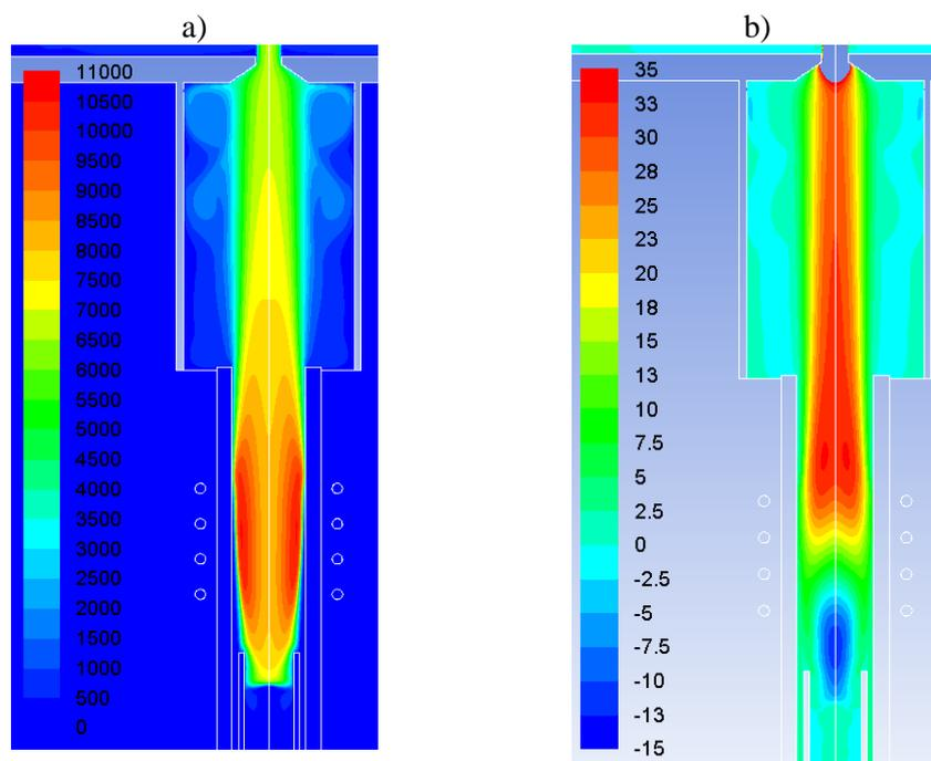
Fig. 5 – Results of calculation for ICP torch (RF power is  $P=30$  kW, coil current frequency is  $f=5.28$  MHz, argon flow rate is  $G=100$  slpm): a – plasma temperature, K; b – axial plasma velocity, m/s
