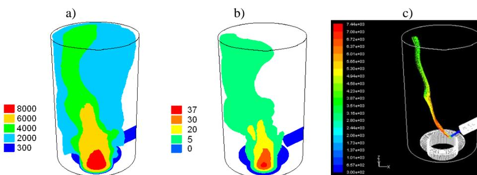
Fig. 7 – Results of calculation of plasma jet with powder feeding (powder feeding rate is 4 kg/h, start velocity is 10 m/s): a – plasma temperature, K; b – axial plasma velocity, m/s; c – trajectory and temperature of  $\text{TiO}_2$  particles with a mean diameter of 15  $\mu\text{m}$  [15]
