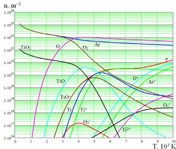
Fig. 2 – Temperature dependence of the composition (species number densities) of mixture of 49.5%  $O_2$  + 49.5% Ar + 1%  $TiO_2$  at 1 atm
