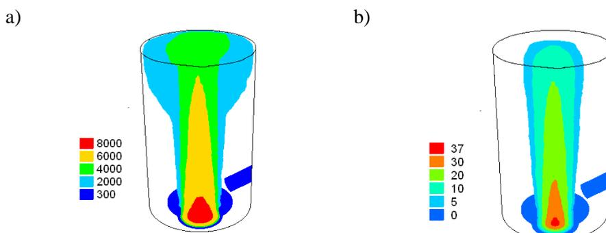
Fig. 6 – Results of calculation of plasma jet without powder feeding: a – plasma temperature, K; b – axial plasma velocity, m/s [15]
