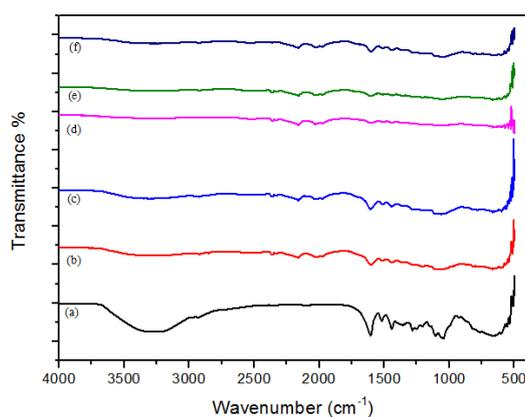
Fig. 3. FT-IR spectra of *Phoenix dactylifera* L leaf extract and as synthesized copper oxide nanoparticles solution with volume ratio a) leaf extract, b) 1:100, c) 1:90, d) 1:70, e) 1:50 and f) 1:30, respectively.
