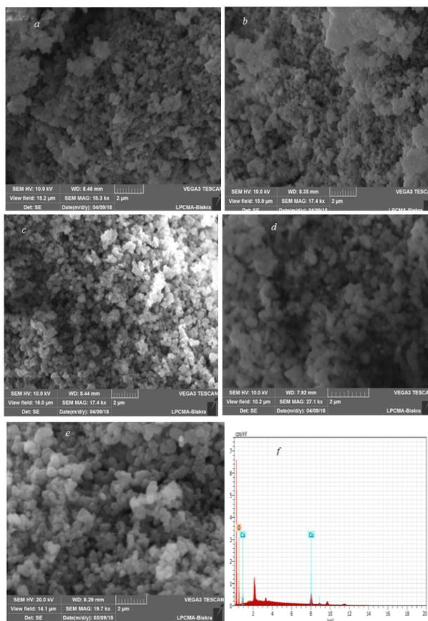
Fig. 6. SEM image and EDAX: (a-e) are SEM images and (f) is the EDAX of copper oxide nanoparticles.
