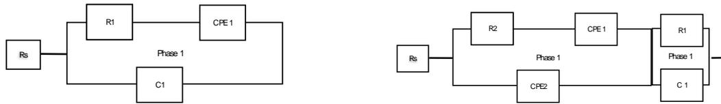
Fig.9 Presenting left T0 fitting circuit and right T1 and T2 fitting circuits
