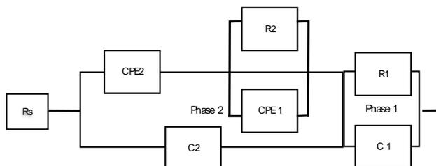
Fig.12 Fitting circuit for Nyquist diagram
