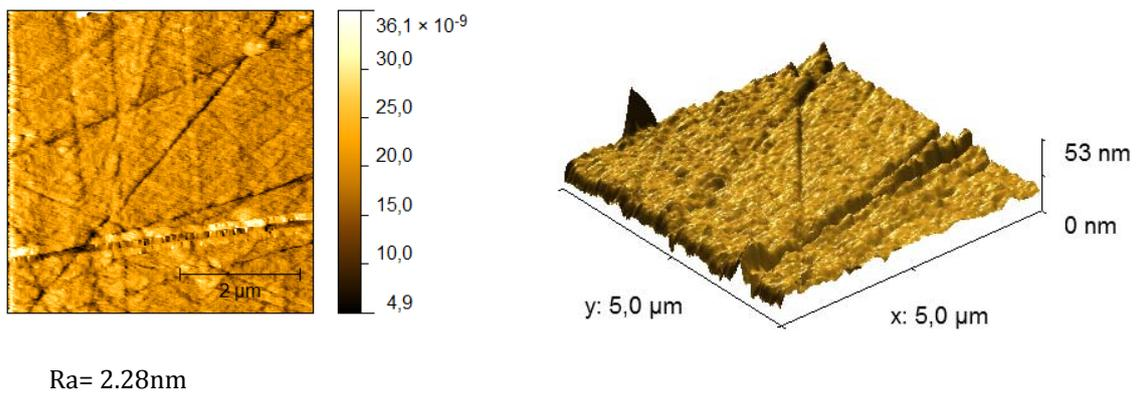
Fig. 4 AFM image of protein layer formation after 30 minutes.
