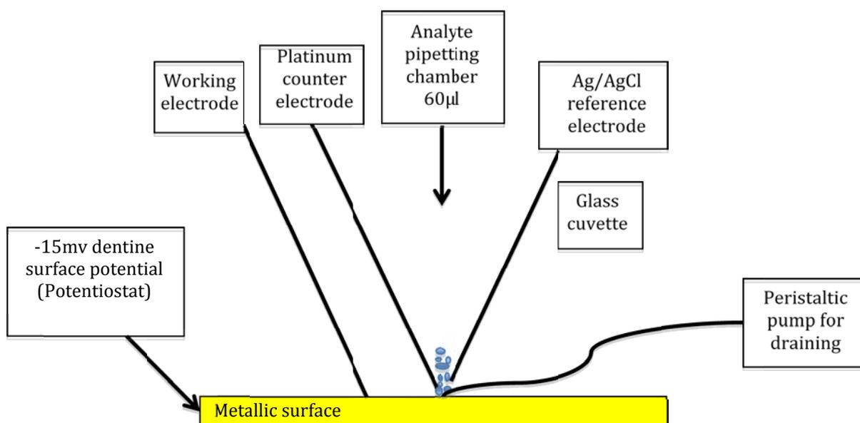
*Fig.2 Diagrammatic representation of custom electrochemical cell used*
