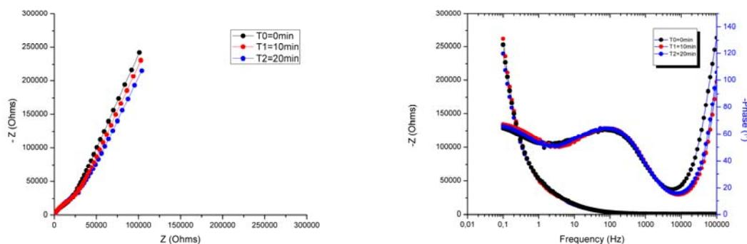
Fig. 3 Nyquist and Bode diagrams showing the formation of the salivary protein pellicle.
