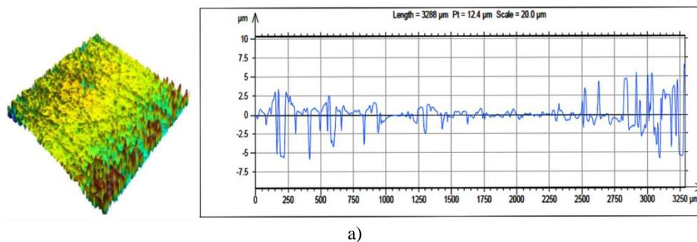
Fig. 5 a) PFDTES-modified polycaprolactone fibrous membrane with roughness value of  $1.52 \mu\text{m}$
