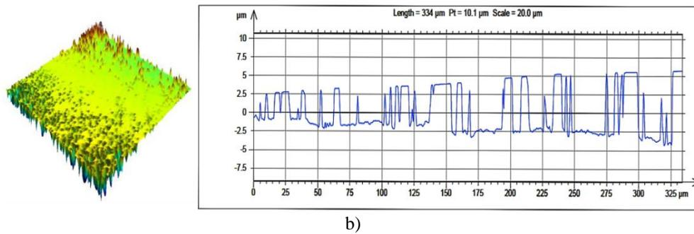
Fig. 5 b), PFDTES-modified polycaprolactone fibrous membrane with roughness value of 1.85  $\mu\text{m}$
