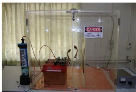
Fig. 1. Electrospinning setup.
