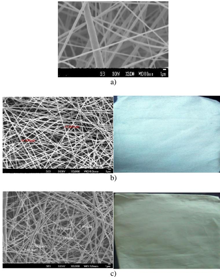
*Fig. 2. Influence of polycaprolactone and PFDTES-modified polycaprolactone solution concentration observed under SEM: a) 15wt%; b) 15wt%; c) 10wt%*
