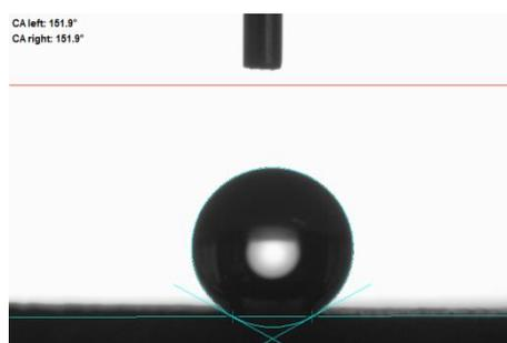
Fig. 7 Super- hydrophobic nature of PFDTES-modified polycaprolactone fibrous after durability test
