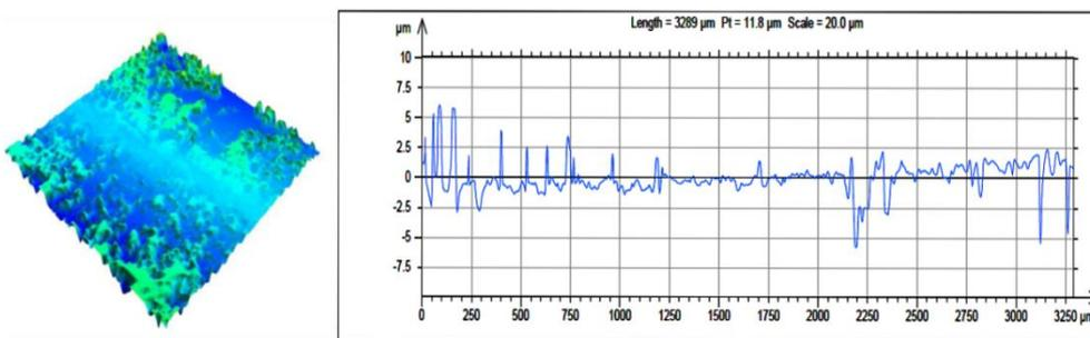
Fig. 6 Without PFDTES-modification roughness value is 0.82 nm
