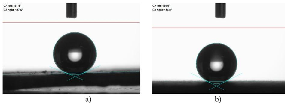
Fig. 4. a) and b) shows water droplet placed on PFDTES-modified polycaprolactone fibrous membrane
