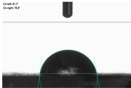
Fig. 3. Water droplet on polycaprolactone fibrous membrane
