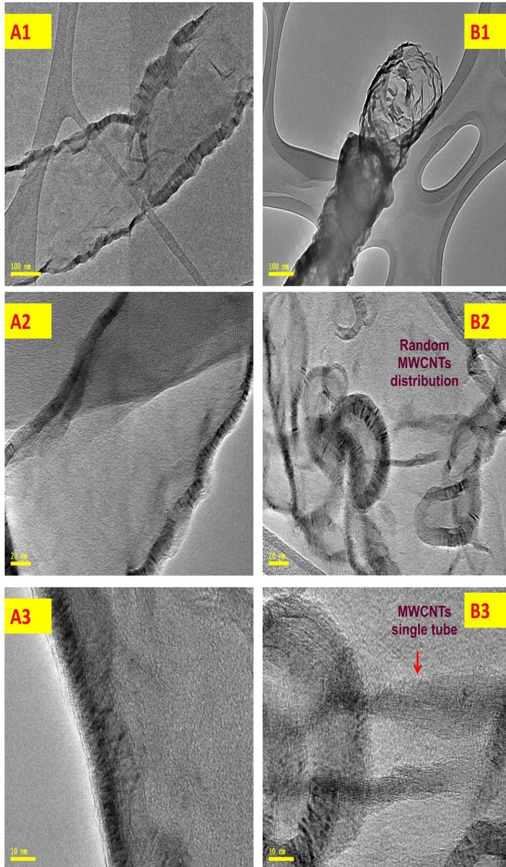
Fig. 2. TEM micrograph of electrospun of PLCL (A1) (A2) (A3) and MWCNTs/PLCL (0.3 wt%) (B1) (B2) (B3) nanofibers at magnification of 100 nm, 20 nm and 10 nm, respectively
