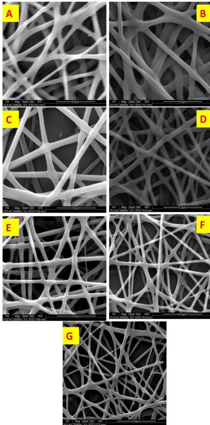
*Fig. 1: SEM micrograph of electrospun (A) PLCL (B) MWCNTs/PLCL (0.1 wt%) (C) MWCNTs/PLCL (0.2 wt%) (D) MWCNTs/PLCL (0.3 wt%) (E) MWCNTs/PLCL (0.4 wt%) (F) MWCNTs/PLCL (0.5 wt%) (G) MWCNTs/PLCL (1.0 wt%) nanofibers*
