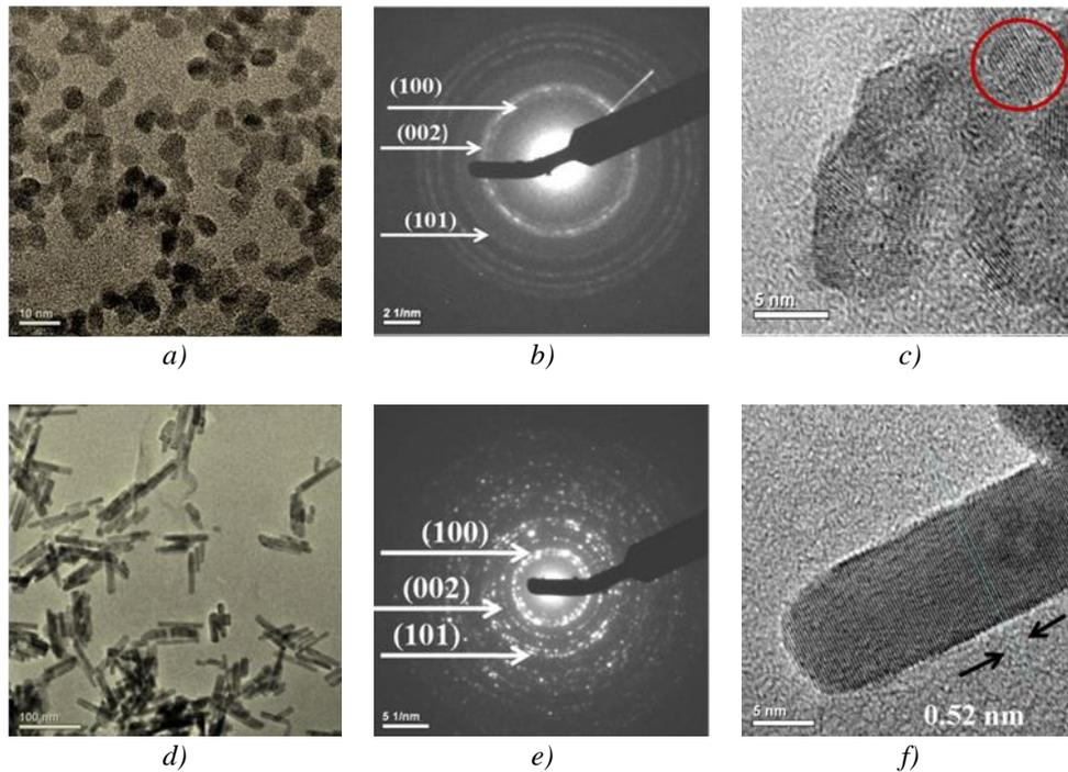
Fig.1. TEM images of ZnO nanostructures. (a) HRTEM of sol-gel nanoparticles disperse in ethanol, (b) corresponding selected area electron diffraction (SAED) of sol-gel NP, (c) image of individual nanoparticles (Lattice image), (d) HRTEM of nanorods disperse in ethanol, (e) corresponding selected area electron diffraction (SAED) of nanorods, (f) image of individual nanorods (Lattice image).
