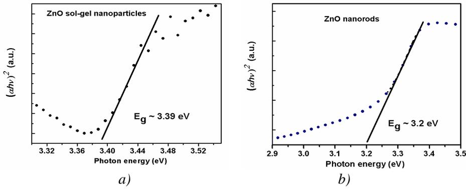
Fig. 3. Tauc plot from UV-Vis analysis of a ZnO, (a) nanoparticles and (b) nanorods that illustrates the fitting of the linear region to evaluate the optical band-gap at the X-axis intercept.
