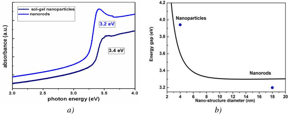
Fig.2. (a). Room temperature UV–Visible absorption spectra near the band edge as a function of photon energy (eV) of ZnO sol-gel nanoparticles and nanorods. (b) Dependence of the lowest excited state vs ZnO nanostructures diameter (solid line). Circles correspond to the optical absorption onsets determined experimentally.
