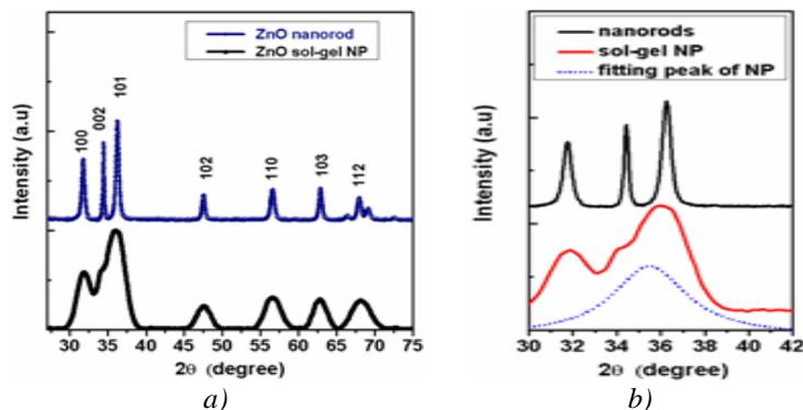
Fig. 1. X-ray diffraction pattern of ZnO nanostructures (a) between  $30^\circ$  and  $70^\circ$  and (b) enlarged view from  $30^\circ$  to  $42^\circ$ .
