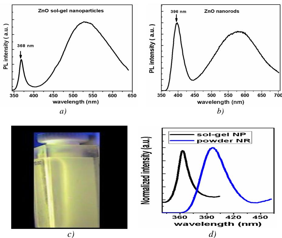
Fig.4. Room temperature steady state PL emission spectra of ZnO nanostructures (a) sol-gel nanoparticles, (b) nanorods, (c) Green luminescence photograph digit of ZnO sol-gel nanoparticles under irradiation with 365 nm ultraviolet light from a UV lamp, and (d) the blue shift of the UV peaks.
