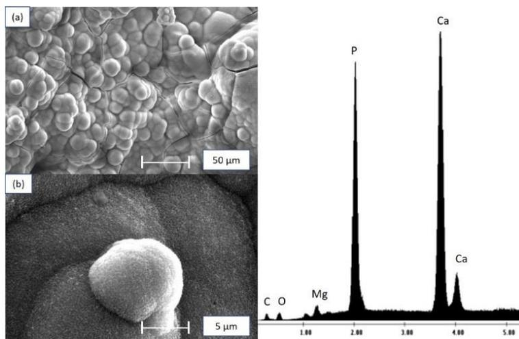
Fig. 4. Micrograph of the specimen (3) of the CO-Cr-Mo alloy coated with HAp, after 21 days of immersion in SBF.
