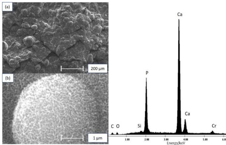
Fig. 3. SEM and EDS of specimen (2) of the surface of the alloy CO-Cr-Mo coated with HAp, after 21 days of immersion in SBF.
