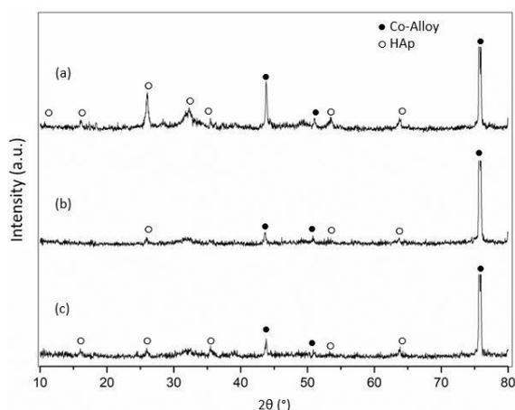
Fig. 1. Diffraction patterns of the metal specimens of the Co-Cr-Mo alloy with the HAp coating, using different parameters of the laser process after being immersed in SBF for 21 days.
