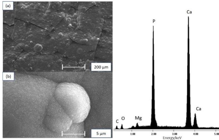
Fig. 2. Micrograph of the surface of the alloy CO-Cr-Mo coated with HAp of the specimen (1), after 21 days of immersion in SBF.
