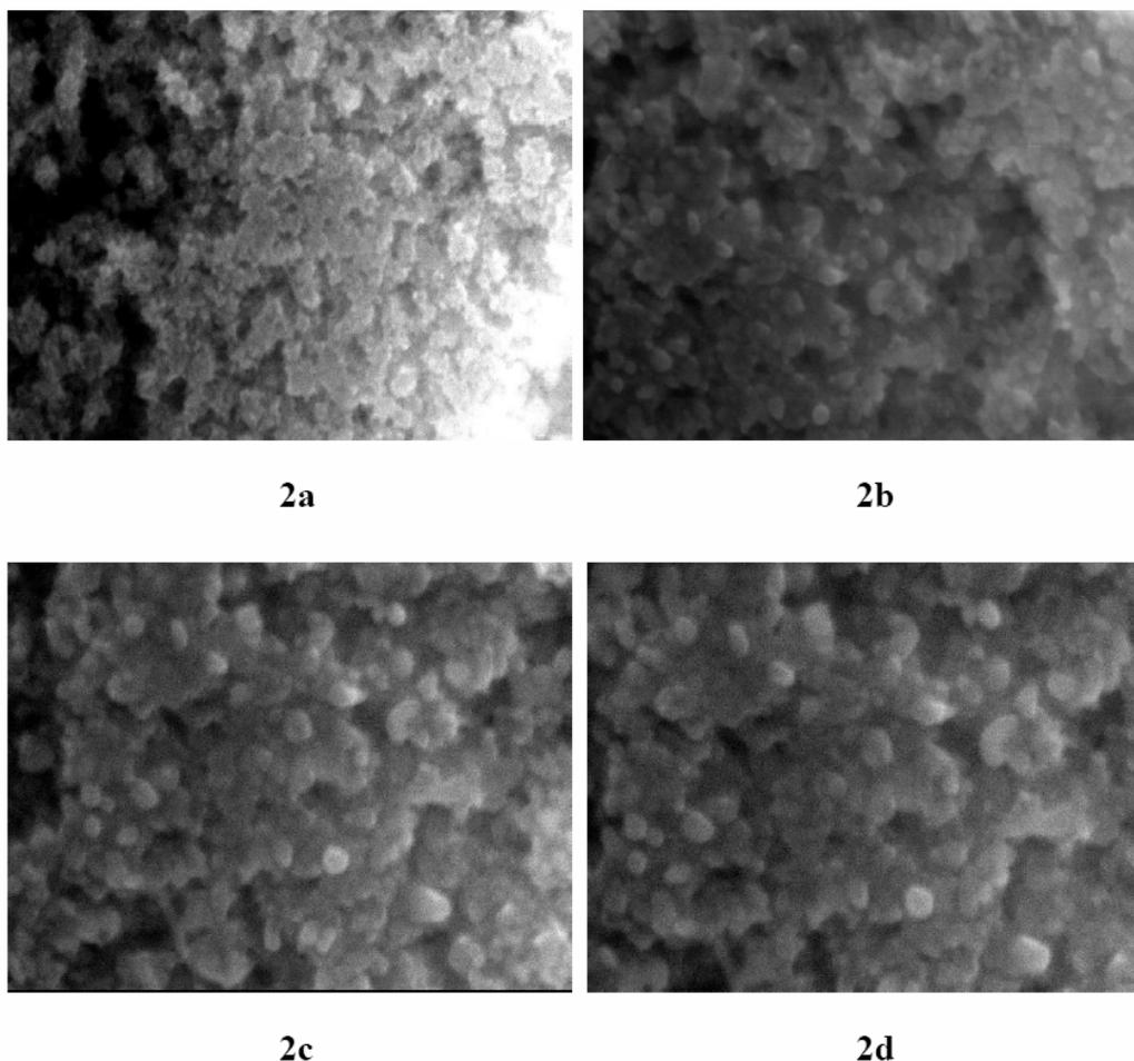
Fig. 2. TEM micrograph 2a(25K); 2b (50K); 2c(60K); 2d(75K) of silver nanoparticles synthesized by the reaction of 1mM silver nitrate with *A.paniculata* antibiofilm extract.
