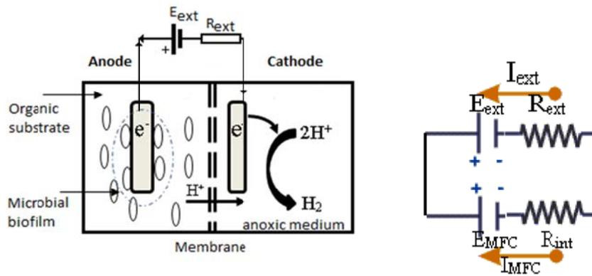
Fig. 2: MEC1 configuration, with negative polarization on the biocathode provided by an external source ( $E_{ext}$ ); protons and excess electrons combine in the anoxic cathode to release hydrogen gas.  $R_{ext}$  is the equivalent resistance of the external circuit; internal resistance  $R_i$  and generated potential  $E_{MFC}$  are shown in the equivalent circuit.
