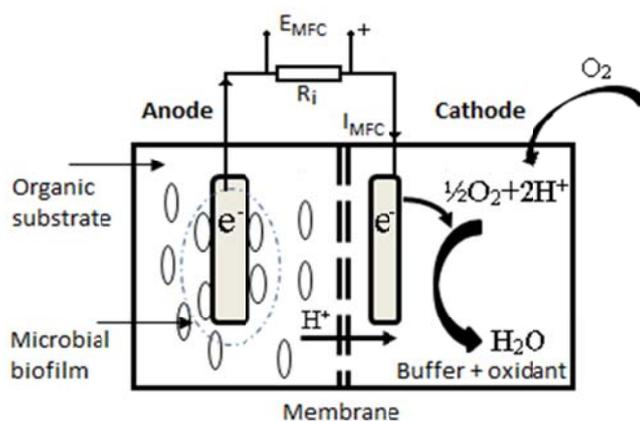
Fig. 1: MFC operation principle. Microbial consortia catabolize the organic substrate, forming biofilms and transferring exoelectrons to the anode; protons migrate through the PEM to combine with oxygen, forming water.  $I_{MFC}$  is the current generated by the MFC,  $R_i$  the equivalent internal resistance and  $E_{MFC}$  the generated potential.
