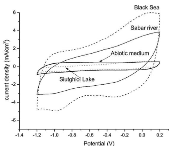
Fig. 4: Cyclic voltammetry for water samples and abiotic medium, at a scan rate of 10mV/s. CVs are recorded after polarization at -1100mV vs. Ag|AgCl for 48h.
