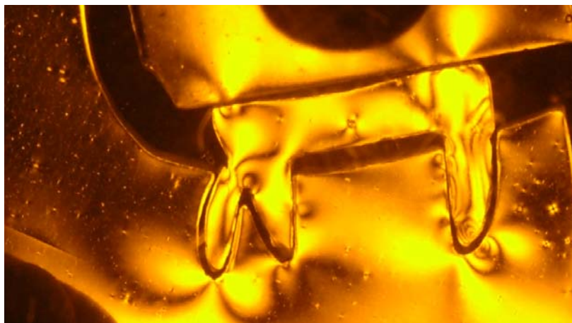
Fig. 8. Model with linear support on two vertical abutments with the load distributed along the whole occlusal surface
