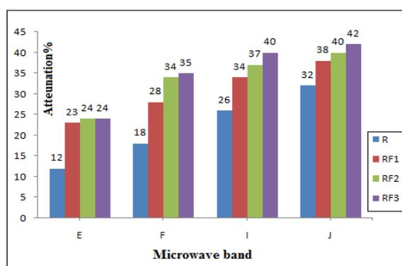
Fig. 7. Microwave attenuation of natural rubber composites.
