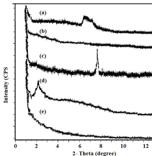
Fig. 4. WXR D diffractograms of a) Na-MMT, b) Na-MMT/PNIPAm, c) Na-MMT/PAMPS, d) Na-MMT/PAMPS-Na and e) Na-MMT/PVP nanogels
