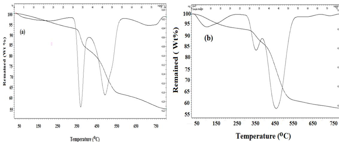
Fig.2. TGA and DTG thermograms of a) Na-MMT/PAMPS-Na and b) Na-MMT/PAMPS nanogels
