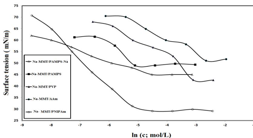
Fig. 5. Relations between equilibrium surface tension of Na-MMT nanogels and their different concentrations at 25 °C.
