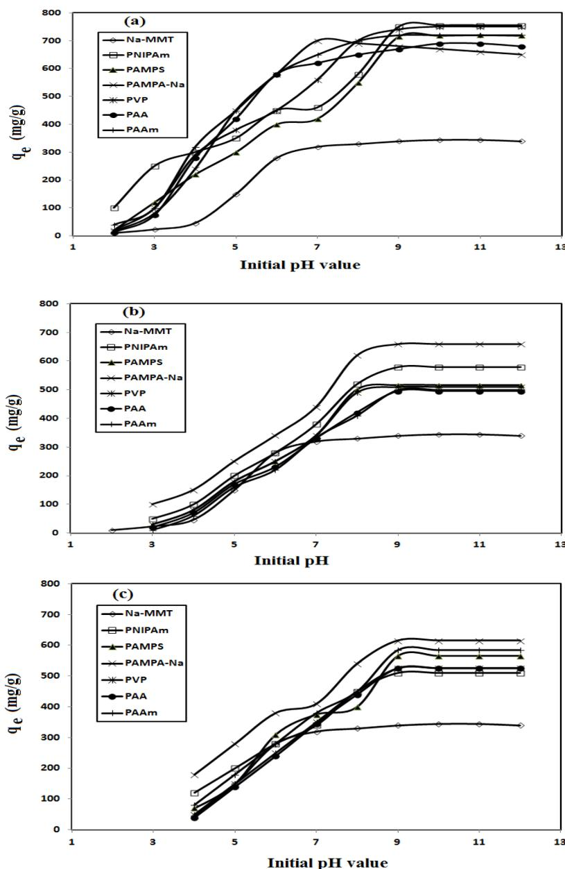
Fig.6. Relation between equilibrium adsorption capacities of Na-MMT nanogels at 1000 ppm in their initial pH of a) MB, b)  $\text{Co}^{2+}$  and c)  $\text{Ni}^{2+}$  aqueous solution at 25 °C.
