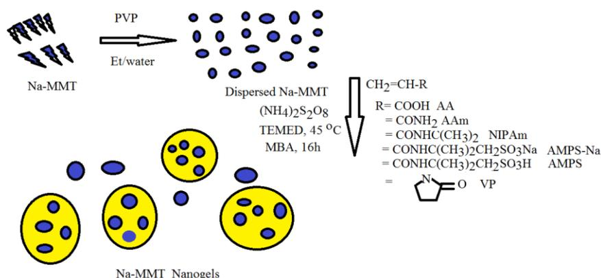
Scheme 1: Preparation of Na-MMT homopolymer nanogels
