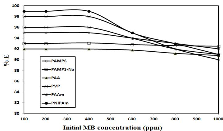
Fig.7. Relation between MB removal efficiencies of Na-MMT nanogels and their different concentrations in aqueous solution at 25 °C
