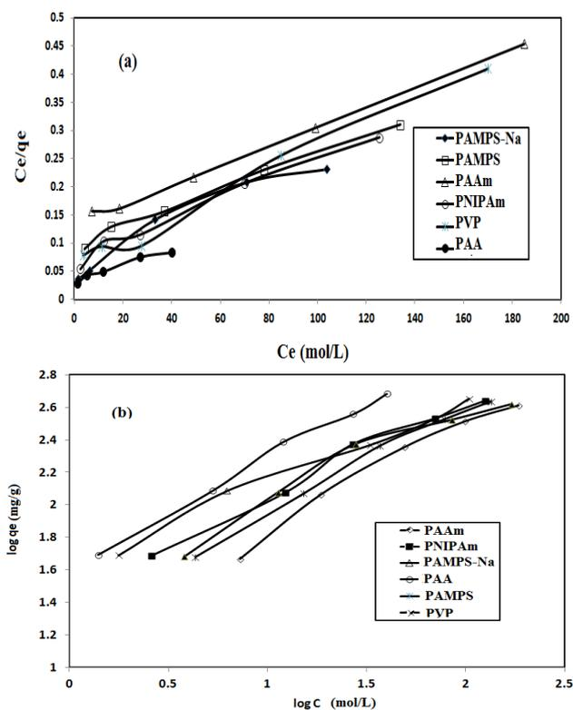
Fig.8. Adsorption isotherms a) Langmuir and b) Freundlich models of Na-MMT nanogels
