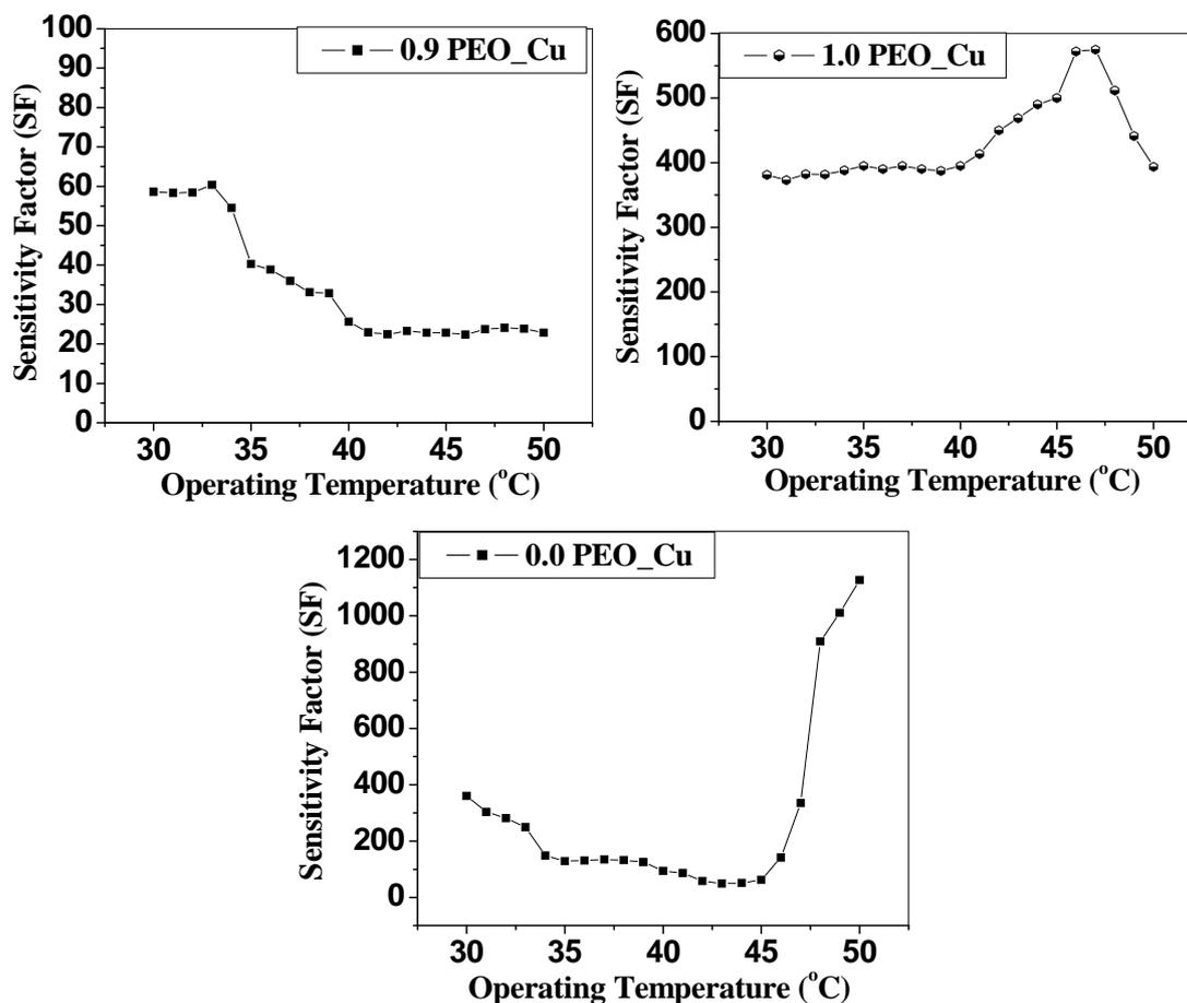
Fig.3 Integrated pictures of operating temperature and Sensitivity of Cu modified PEO with 0.9, 1.0, 0.0 additive concentrations
