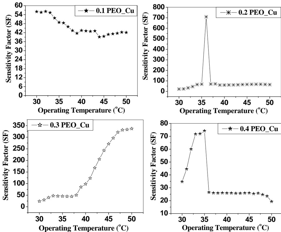
Fig.1 Integrated pictures of operating temperature and Sensitivity of Cu modified PEO with 0.1, 0.2, 0.3, 0.4 additive concentrations
