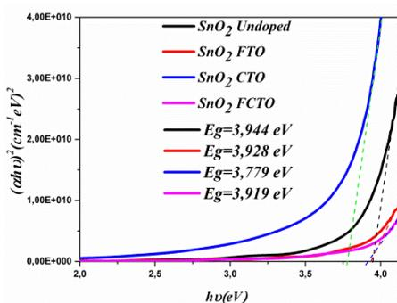
Fig. 2. Band gap ( $E_g$ ) estimation from Tauc relation of undoped tin dioxide, F doped (FTO), Co doped  $\text{SnO}_2$  (CTO) and F-Co co-doped  $\text{SnO}_2$  (FCTO) thin films.
