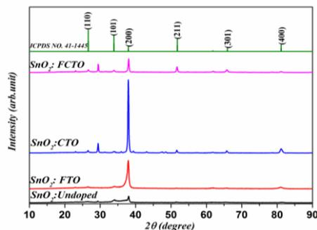
Fig. 4. XRD patterns  $\text{SnO}_2$  images of undoped, F doped  $\text{SnO}_2$ :(FTO), Co doped  $\text{SnO}_2$ :(CTO) and F-Co co-doped  $\text{SnO}_2$ : (FCTO) thin films.
