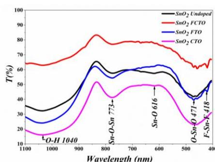
*Fig. 3. FT-IR spectra of undoped, F doped SnO<sub>2</sub>:(FTO), Co doped SnO<sub>2</sub>:(CTO) and F-Co co-doped SnO<sub>2</sub>: (FCTO) thin films.*
