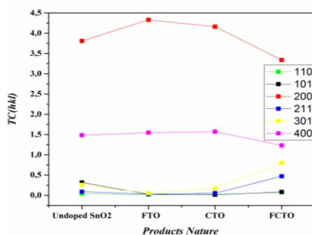
Fig. 5. TC (hkl) variation of undoped, F doped  $\text{SnO}_2$ : (FTO), Co doped  $\text{SnO}_2$ : (CTO) and F-Co co-doped  $\text{SnO}_2$ : (FCTO) thin films.
