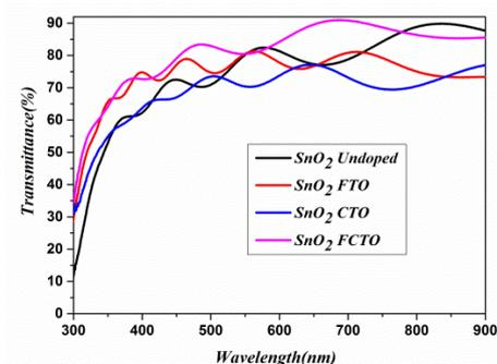
Fig. 1. Transmittance spectra of undoped, F doped  $\text{SnO}_2$ :(FTO), Co doped  $\text{SnO}_2$ :(CTO) and F-Co co-doped  $\text{SnO}_2$ : (FCTO) thin films.
