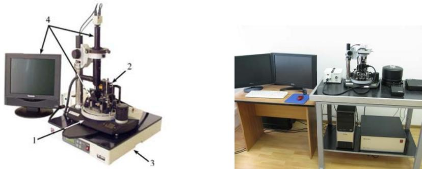
Fig. 2. AFM Microscope, NTEGRA Probe NanoLaboratory NT – MDT. a) 1 – base unit; 2 – measuring head; 3 – vibrations isolation system; 4 – optical viewing system.
