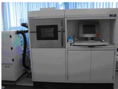
Fig. 1. Selective laser sintering machine (rapid prototyping) EOS M 270 Titanium Version
