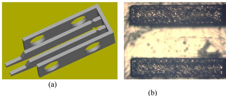
Fig. 3. Microgripper produced using EOS M 270 Titanium Version laser sintering system.
