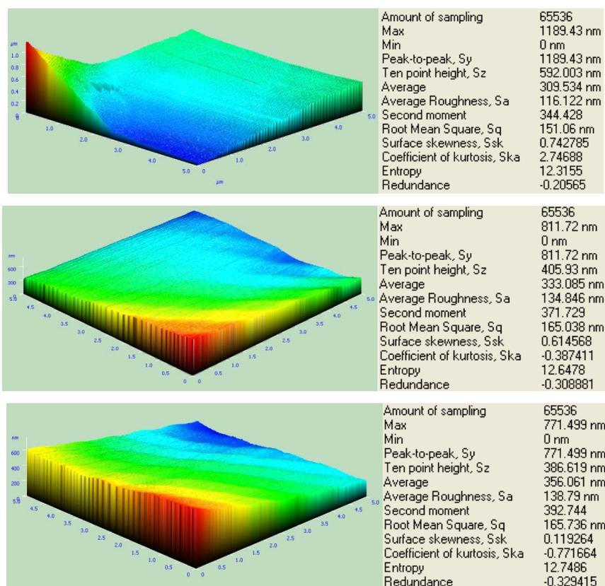
Fig. 4. Roughness of microgripper's surface measured using NTEGRA Probe NanoLaboratory
