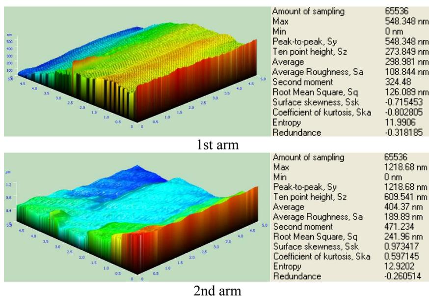
Fig. 5. Roughness of microgripper arms surfaces measured using NTEGRA Probe NanoLaboratory
