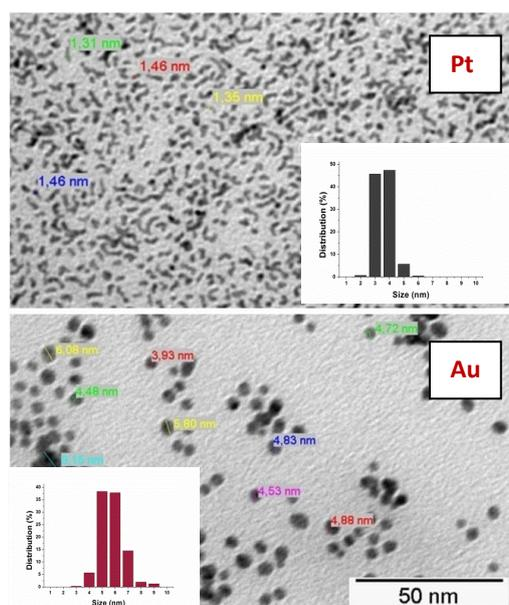
Fig. 2. TEM images of AuNPs and PtNPs sputtered into PEG after deposition diluted with water in ratio 1:9 with inset figure of size distribution histograms.
