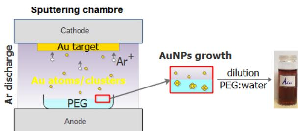
Fig. 1. Principle of AuNPs solution preparation by direct sputtering into liquid (PEG).
