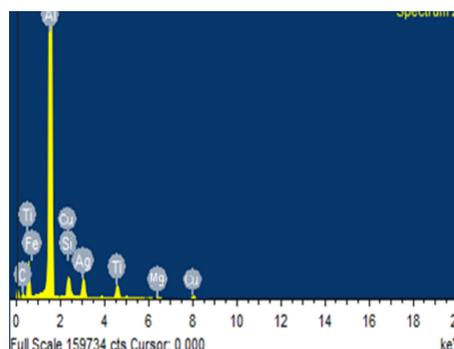
Fig. 2. EDS graph of A356 + SiC + Gr.
