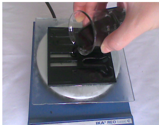
Fig.3 Dispersion of MWCNTs in polyester matrix under oscillating magnetic field
