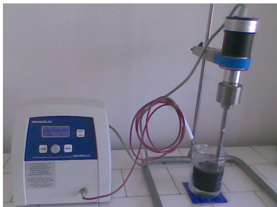
Fig.2 Ultrasonication of MWCNTs suspension using BANDELIN HD3200 generator
