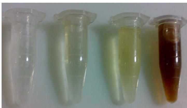
Fig. 1. Color change of silver nitrate 1mM solution from colorless to yellow-brownish as the reaction proceeds on addition of the culture supernatant *Enterobacter aerogenes*.
