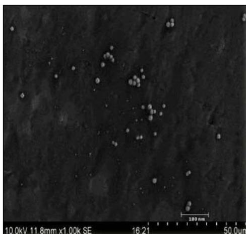
Fig.3. SEM micrograph of the silver nanoparticles( scale bars correspond to 50  $\mu\text{m}$ ).
