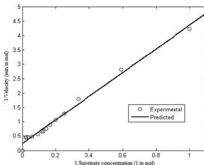
Fig. 8. Lineweaver-Burk plot of kinetic data, showing the significance of the axis intercepts and gradient.
