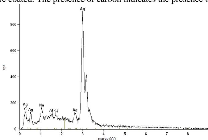
Fig.5. EDX spectrum of silver nanoparticles.
