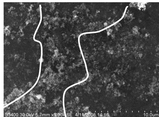
*Fig. 3 thermal conductive channel of composite*
